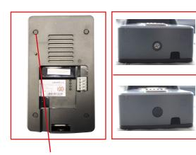
9. Put the screw cap covers in place over the screws at the back of the smartbell. Attach the smartbell to the bracket. Secure the unit to the bracket using the provided screw and place at the bottom of the unit. Then use the cap to cover (shown above, right).
