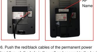
lead through the hole in the wall and connect to the back of the smartbell. The red wire into the number 1 slot and black into the number 2 slot. To do this, push and hold the grey clip in while pushing in the red//black cables. When pushed in, release the clip to secure the wire.
