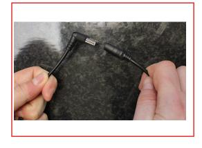
4. Take the permanent power lead and plug it into the DC plug on the power supply provided. Please DO NOT plug the power supply into your power source at this point.
