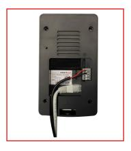
7. If you choose a wired connection to your router/home plug/switch, run your ethernet cable through the hole and connect to the back of the smartbell. Attach as shown above. If you choose a wireless connection skip this step and proceed to step 6.
