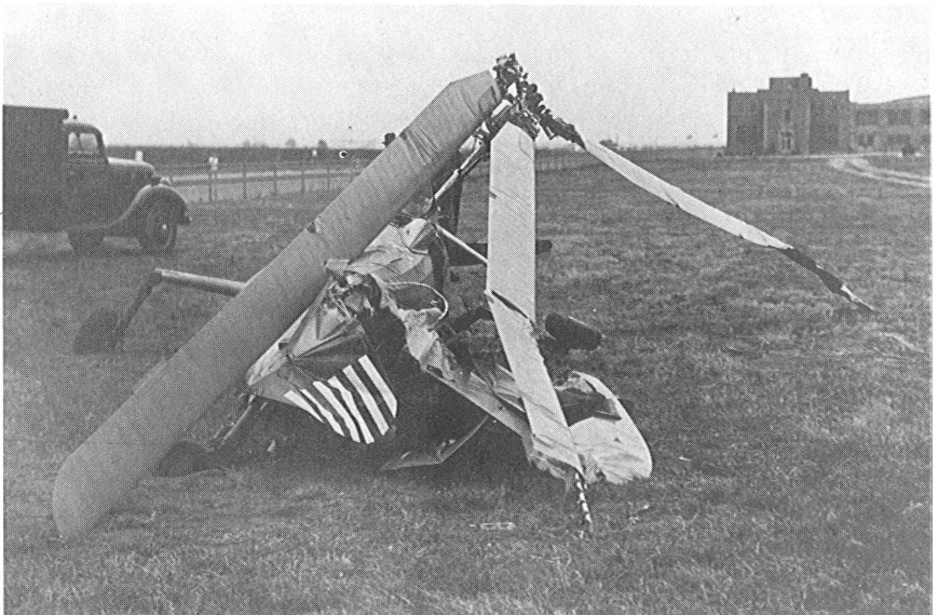
Figure 2. The Kellett XR-2 Autogyro Before and After Ground Resonance.
