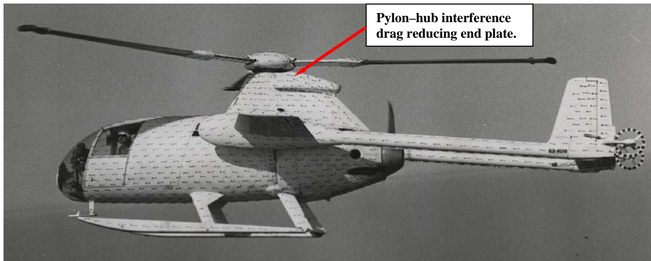
Figure 14. Early XV-1 Flight Testing Was Devoted to Drag Reduction, the Major Problem Hohenemser Repeatedly Identified During the Full Scale Wind Tunnel Testing.
