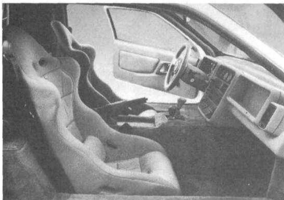
THE interior of the RS200 uses a number of current Ford components yet still manages to look distinctive. Note the two (Sierra) transmission control levers, the taller operates the five-speed gearbox while the shorter selects the required torque split to the front wheels.
