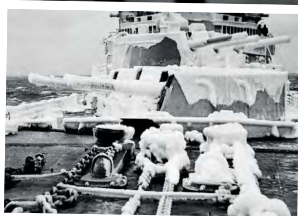
LEFT Some of the ice that formed on HMS Belfast's 'A' and 'B' gun turrets during the winter of 1943.
