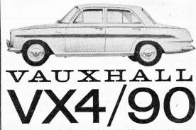
1.5 litre 4-cylinder engine. 81 bhp at 5,200 rpm. Aluminium cylinder head. Twin carburettors. Special inlet manifold. 4-speed all-synchro gearbox, short floor-mounted lever. Power assisted brakes, discs at front. Specially tuned suspension for fast, tough driving. Lubrication every 30,000 miles.
