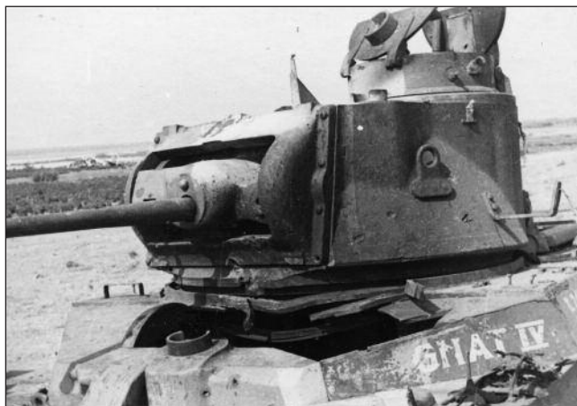
Left: Gnat IV was struck just below the gunsight where the base of the mantlet meets the turret. The resulting explosion blew off the driver's hatch and part of the hull roof armour and warped the turret ring. The blackening of this area of the turret and hull is consistent with the Australian observation that the tank appeared to catch fire. Note the Junkers Ju 52 wreck behind the tank, one of the over 280 transport aircraft lost by
