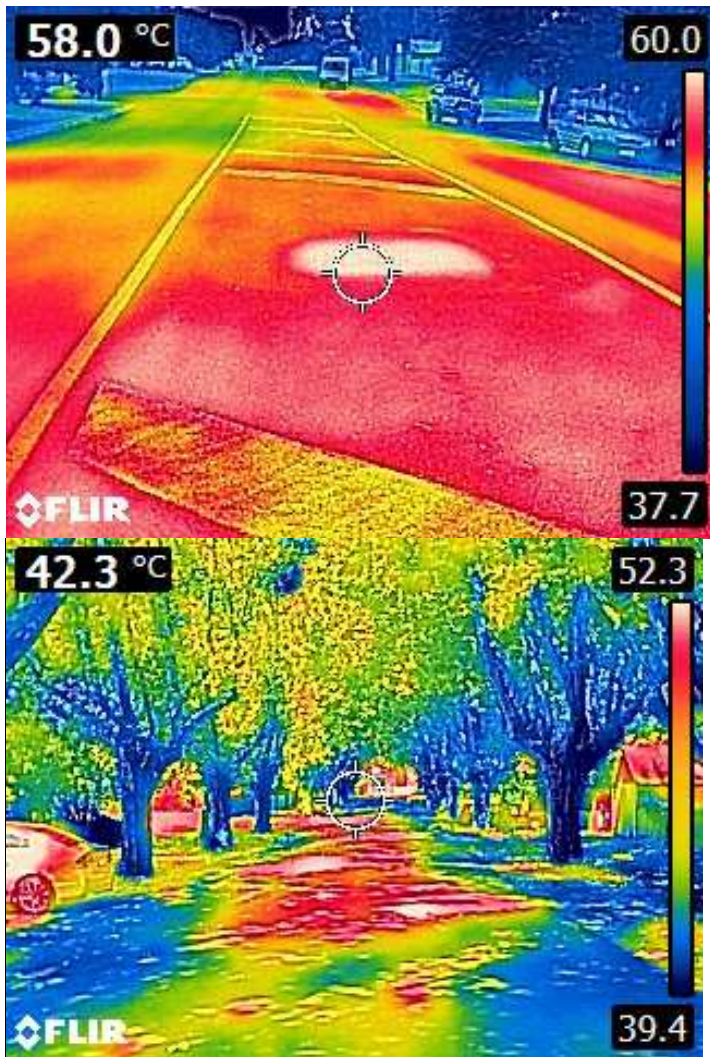
Figure 5. Two thermal images taken in Bendigo in January 2019 demonstrating the effect that street trees have on cooling the surrounding streetscape. Brougham Street is shown on the left; Marks Street on the right.
