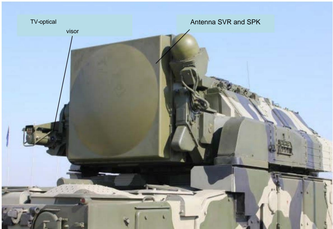
Rice. 5. Target tracking and missile guidance station (SVR and SPK) and backup television optical sight
