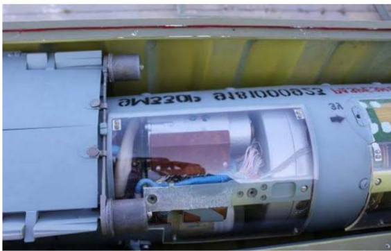
The second compartment is the control compartment
