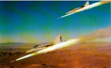
Upgraded Zuni missiles on. The 127 U.S. Marine Corps F/A-18D is commonly used by the U.S. Navy Marine Corps F/A-18D to mark targets as part of the Fleet Air Support (Forward Air Controller) mission. To increase the on-the-ground level, Zuni missiles can be equipped with a variety of head types, including anti-explosive, anti-vehicle, color, incendiary and day/night. The pod most commonly used to launch these missiles is the four tube LAU-10 pod, a 48mm construction made of impregnated paper with an aluminum outer covering.
