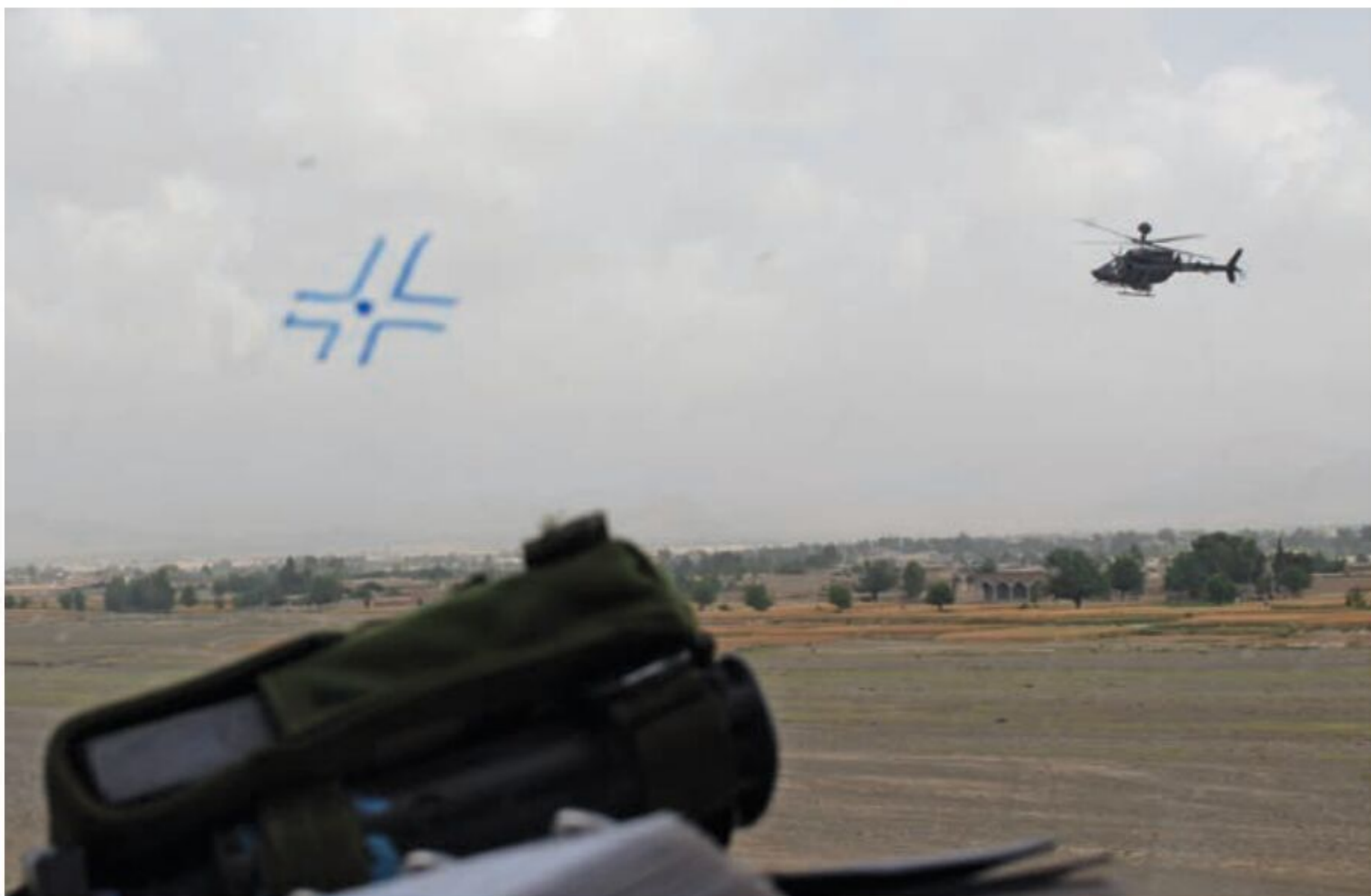
Above: It's not high-tech, but it worked. Known formally a Ballistic Area Reference Point, the OH-58D pilots' "pipper" was actually a dot they made by hand with a dry erase marker on the helicopter's forward canopy glass. Here's Priester's aiming reference as seen from the cockpit. (Photo courtesy Joseph Priester)
