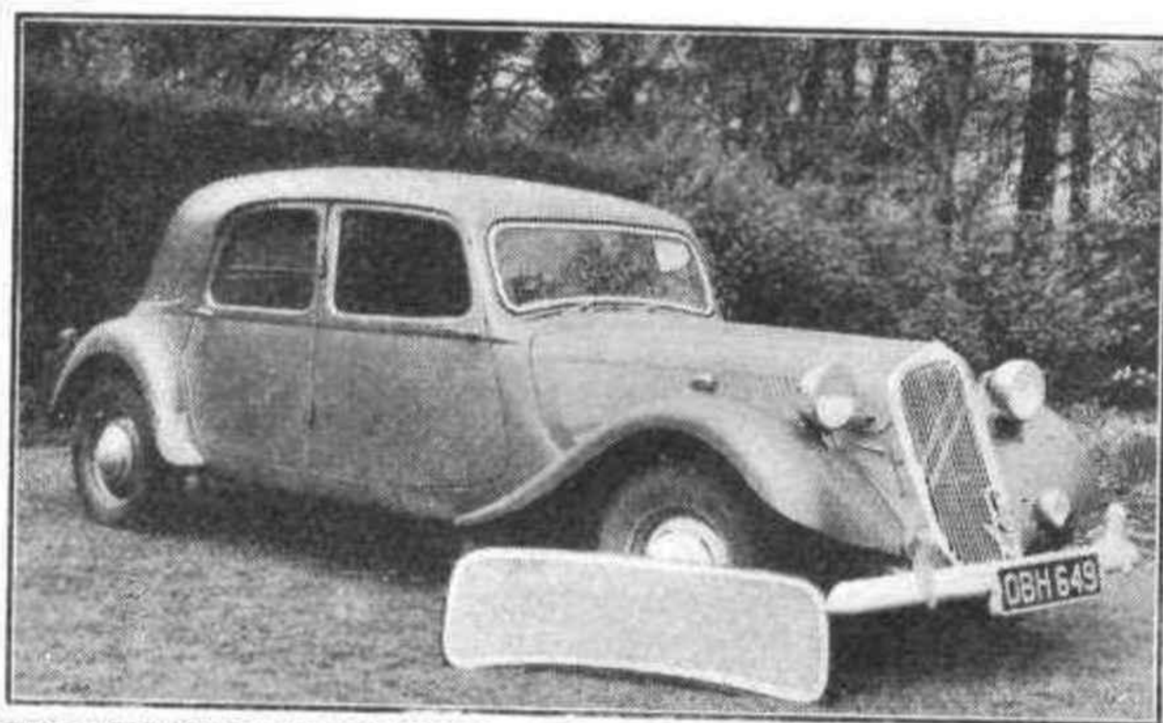
TOUGHENED TROUBLE. —This untouched photograph shows how little could be seen through the windscreen after a stone had struck it—note that you cannot see the wheel and tyre behind it, and then compare with the replacement screen, expeditiously fitted for us by Citroën.
