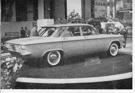
CAR OF THE SHOW is the Chevrolet Corvair, powered by an air-cooled flat six engine mounted at the rear. Allround independent suspension is employed.
