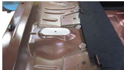
Hot melt access panel under rear seat base
