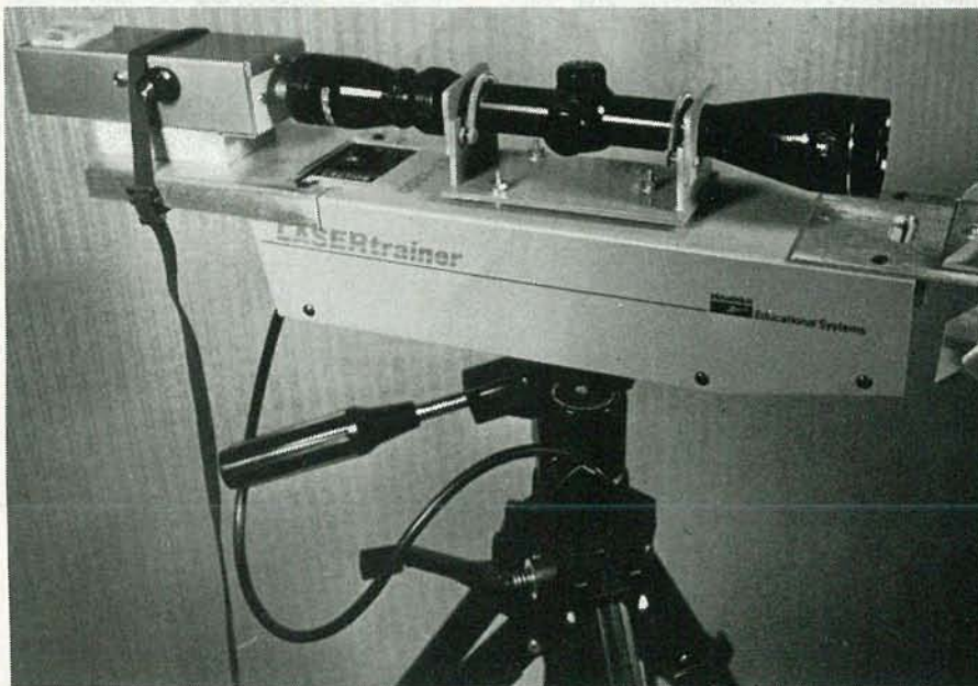
FIG. 2—FOR LONG-RANGE USE the laser and the receiver should be combined into an integral unit so both are aimed together. The telescopic signal provides precision aiming on the target.
