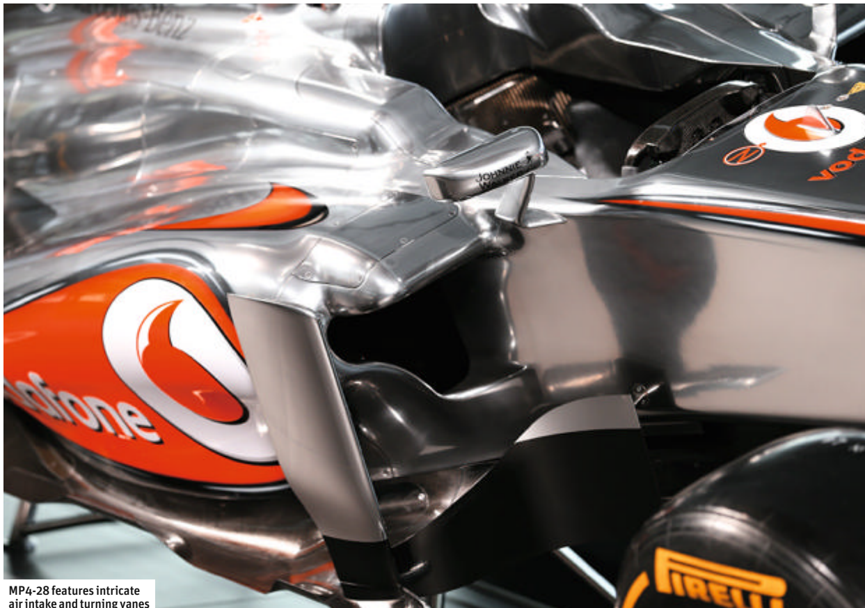
Undercut sidepods will help rear-end aero gains
