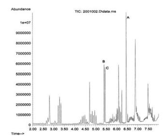
**Figure 1.** Full scan TIC of certified organic geranium oil spiked with methylhexaneamine. Peak A: Internal Standard, Peaks B: and C: the two isomers of methylhexaneamine.
