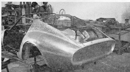
SHAPELY TAIL (left) of a GTO. The car's framework has been completed and the bodywork fitted over it and welded together. Note the hammer marks on the metal and the beautiful welding.
