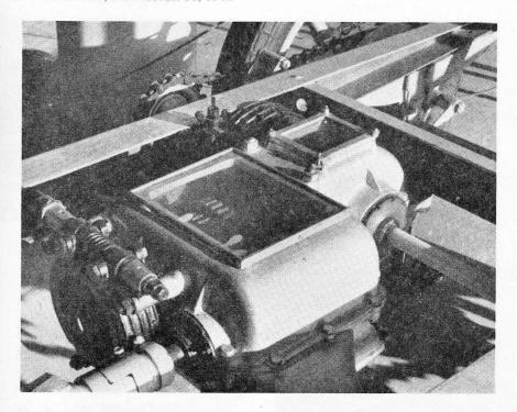
INSPECTION of the chassis of a 1908 Fiat reveals the transmission, which is still by side chains. A glass cover has been fitted to the gearbox so that the innards may be viewed.
