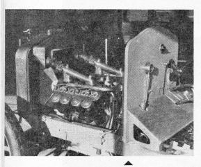
FOUR-LITRE V8 engine of the 1911 De Dion. The side-valve unit features fixed heads and screwed-in valve caps—the valve springs are enclosed, and the induction passages are minute.
