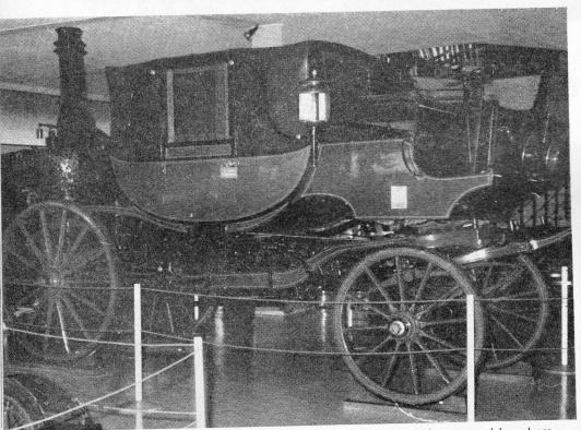
BEAUTIFULLY RESTORED is the 1854 Bordino coach, which is powered by a large twin-cylinder horizontal steam engine driving directly on to the rear axle which is, in effect, the crankshaft. It ran at 5 m.p.h. under favourable conditions.
