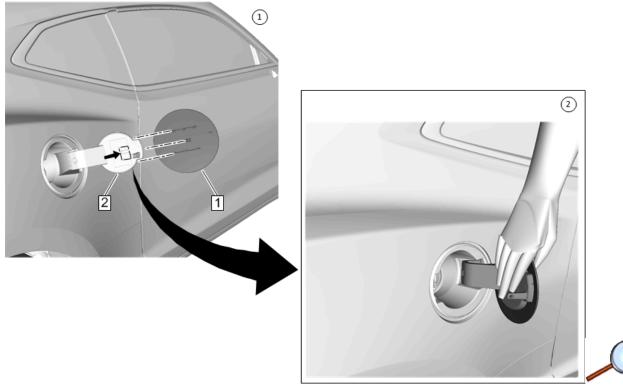
3. Position accessory door (1) along door hinge (2) using same sliding motion to re-install the door onto the hinge. Pressure may need to be applied to engage the door tabs to the hinge tabs before sliding the door to its final install position.
