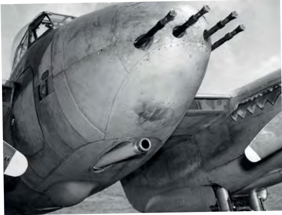
Above Molins six-pound cannon in the nose of a Mosquito XVIII.
