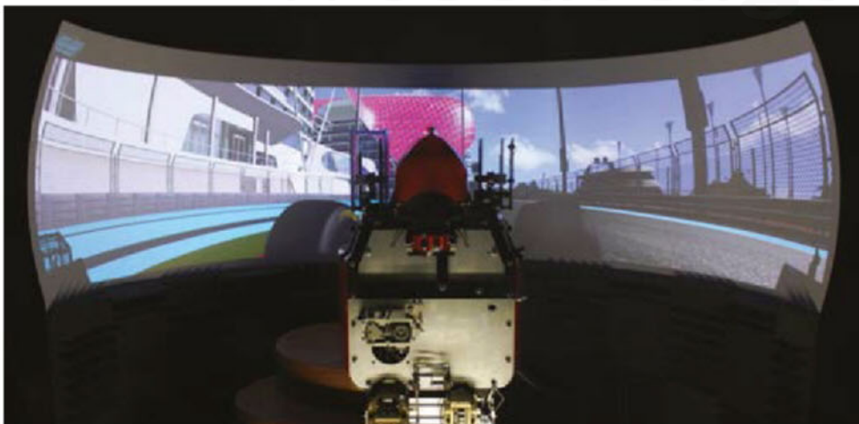
Another example of a static simulator from Pro-Sim which focused on the most important cue of the driver: the visuals
