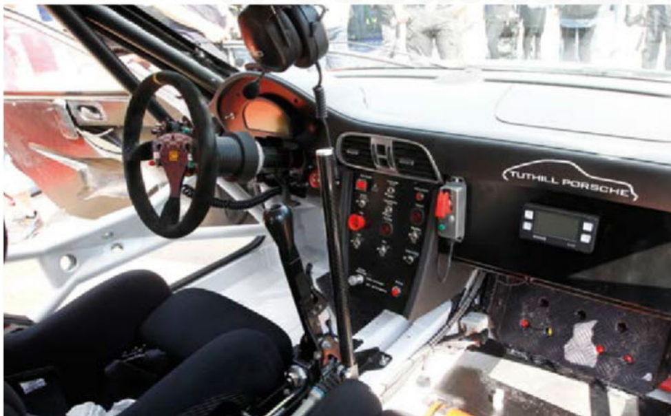
The car contested Rally Germany using Carrera Cup gear ratios and final drive. Graham Moore says: 'We didn't use sixth gear but the engine did have a reasonable amount of torque and we would look at the ratios in conjunction with the restrictor'
