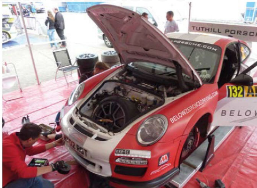
With a front-mounted spare and a fuel tank up-front the static weight balance has been brought forward
