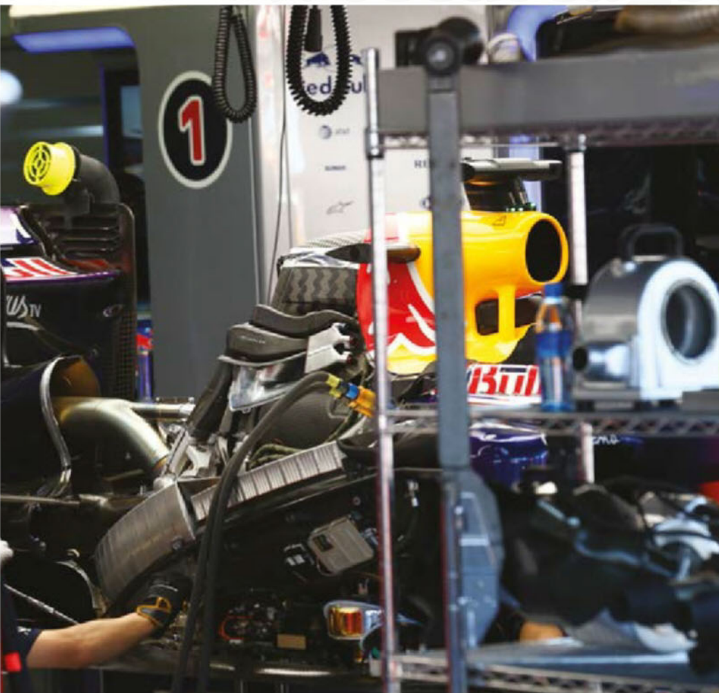
The narrow and long PWR heat exchanger sits above the intercooler, contrary to popular belief the RB10 does not suffer from cooling issues.
