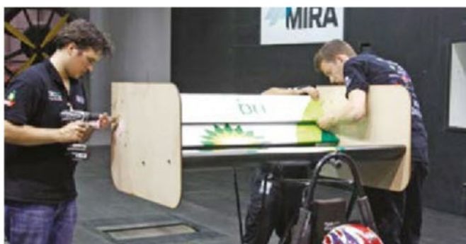
Figure 3: New rear end plates facilitated lower flap angles to be tested
