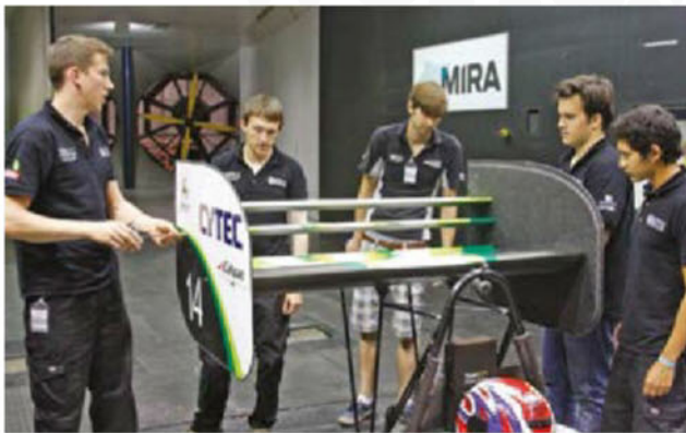
Figure 5: 'Low drag' mode for the acceleration test
