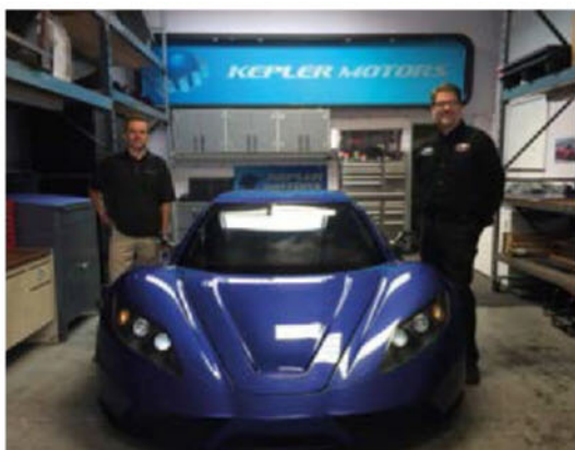
The Motion sits on a carbon-fibre composite monocoque chassis and body, F1-style double wishbone, and pushrod suspension with cast titanium uprights
