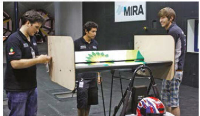
Figure 6: Rear wing in the first dual-element configuration
