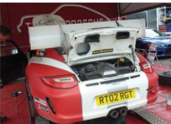
With the flat-six power train rearwards of the rear axle line, the R-GT's weight remains rear-biased
