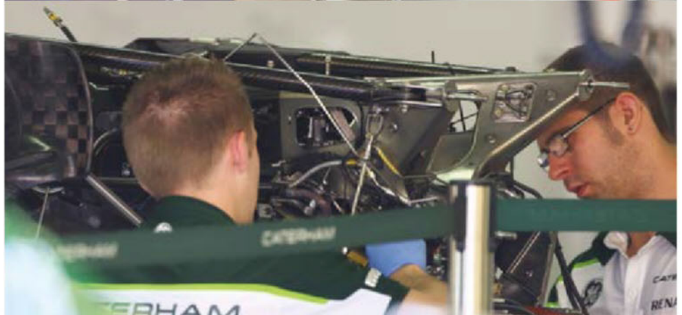
Red Bull developed two transmissions for the 2014 season, one for the RB10 (top) and the other for the Caterham CT05 (above). The forward section of the first iteration of the latter is believed to have had to be reworked due to its tendency to catch fire, while the former features a metal forward section which did not suffer from similar issues.
