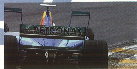
The sidepod-mounted X-wings give greater downforce on the twisty circuits
