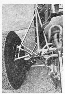
REAR SUSPENSION details are visible here, also the gear-change mechanism of the Colotti-Francis gearbox.
