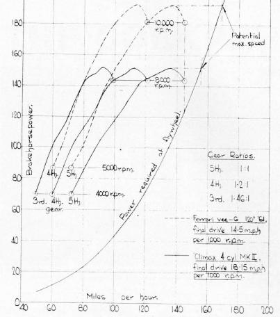
Fig. 1 The Ferrari V6 120-degree, and Mk. 2 Coventry Climax 4-cylinder power curves, compared with the suggested common power requirement curve of the Ferrari, the 1961 Cooper, and the 1960 Lotus.
