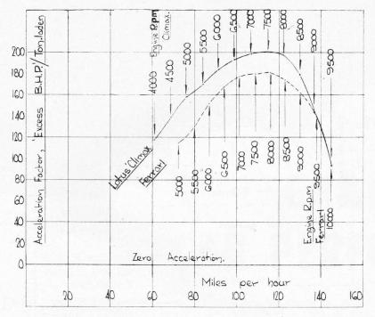
Fig. 3 A direct comparison of the Ferrari and Lotus 24 acceleration potential, produced by division of "excess power" values by the respective vehicle weights.
