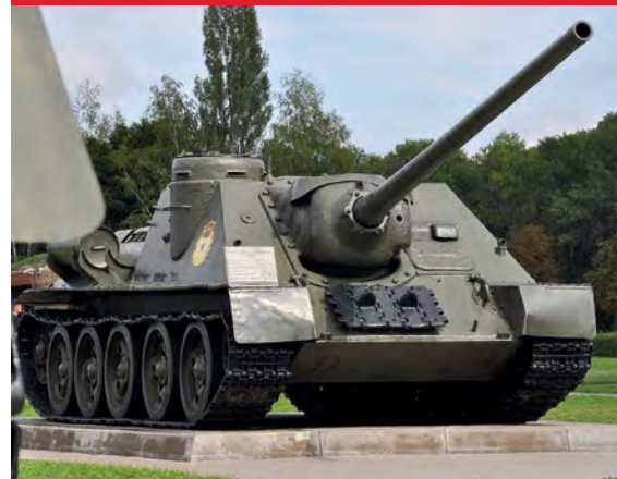
An SU-100 self-propelled gun The SU-100 was the last such wartime weapon, replacing the Kursk era SU-85 Though labelled as self-propelled guns, the primary role of these vehicles was as long-range tank destroyers
