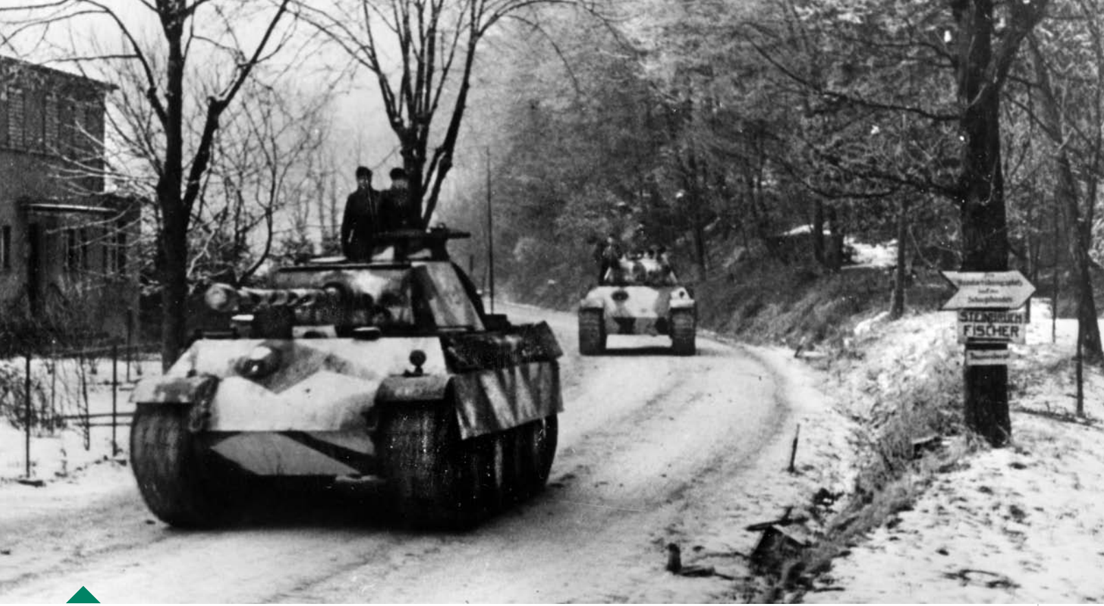
German PzKpfw. V Panther medium tanks, mounting high-velocity 75 mm cannon, advance along a snow-covered road in the Hagenu Forest and the lower Vosges Mountains of France on January 31, 1945.
