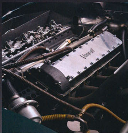
The powerful 2.5ltr Vanwall engine pumped out up to 285bhp at 7,500rpm, depending on what fuel was in the tank
