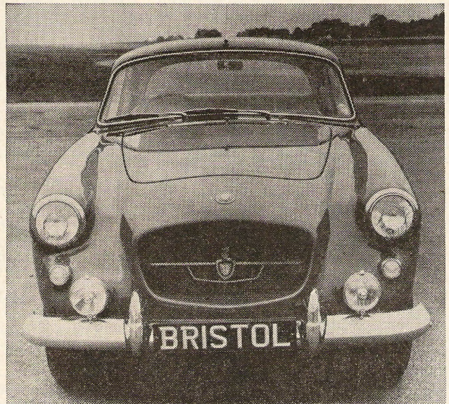
★ FIVE-POINT-TWO: The new Bristol 407 with a Chrysler 5.2-litre V-8 engine and "push-button" Torque-Flite automatic transmission. It will be introduced at this year's Motor Show with a price tag of £5,141 17s. 3d. (inc. P.T.). Power output of the 5,130 c.c. engine is 250 b.h.p. at 4,400 r.p.m. ★
