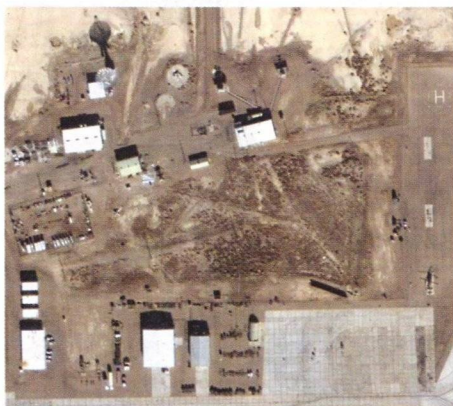
Towards the north of the main Groom Lake base area are three helipads for the airfield's security helicopters. A single HH-60G Pave Hawk can be seen parked there in this view. Above that are the DYCOMS (Dynamic Coherent Measurement System, a radar cross-section measurement system for the development of Stealth technology) and Quick Kill radar systems and various support buildings. DigitalGlobe
