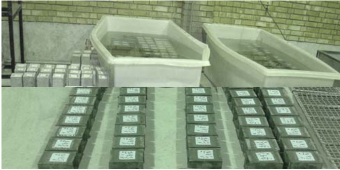
Fig. 2. Manufacturing and curing of cubic samples
