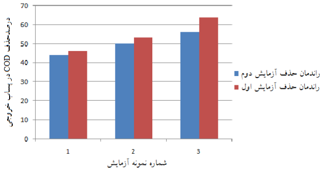
Fig. 7 Compares the effluent COD removal efficiencies of the two tests
