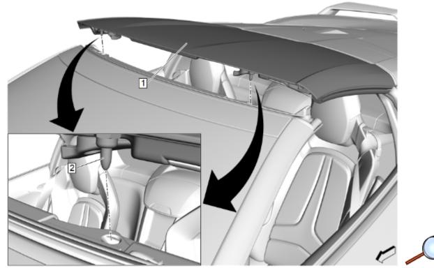
4. Lift the front of the roof lift off panel (1) to disengage the roof lift off panel locating pins (2).
