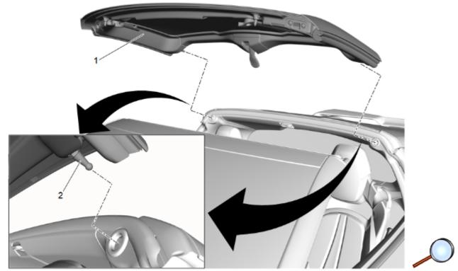
1. Slide the roof lift off panel (1) rearward to engage the roof lift off panel locating pins (2).
