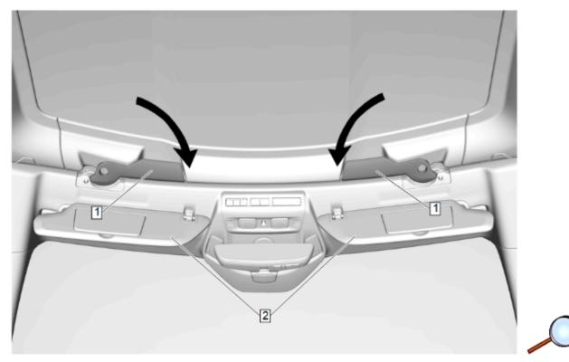
**Note:** There will not be an audible click, but the latches will firmly fit in place by detent. 4. Rotate the roof lift off panel/window latch handles (1) inward until full travel is reached.
