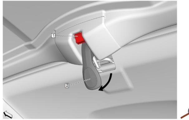
1. Depress the rear latch release button (1) and rotate the roof lift off panel/window rear latch (2) down and forward, ensuring the latch clamp has released.
