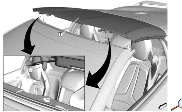
2. Gently lower the roof lift off panel (1) and engage the roof lift off panel locating pins (2).
