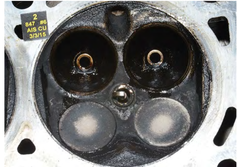
Cylinder Head After Cleaning with CRC 05319
