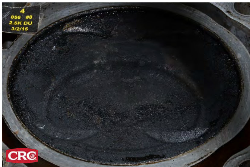
Piston Top (Dirty) Carbon Deposit Thickness in Mils = 4.59
