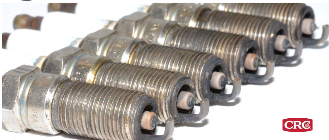
Spark Plugs After Cleaning with CRC 05319
