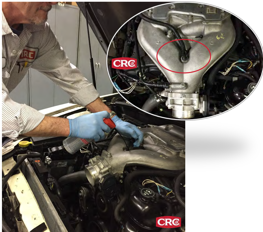
Or professionals can spray through a vacuum line connected to the intake manifold (i.e. brake booster vacuum line)
