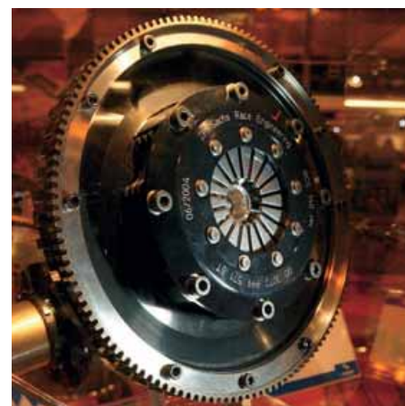
Below right: also from ZF Sachs came this detachable racing flywheel for GT racing Porsches that can be disengaged after start-up, massively reducing the rotational mass of the engine
