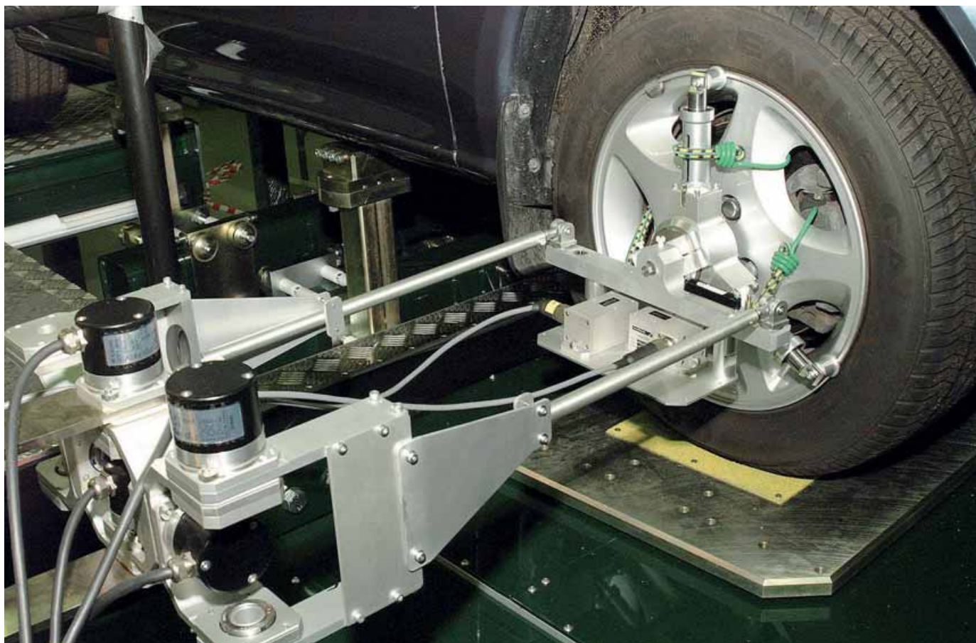
The Lotus rig measures the movement of each wheel in all directions – three translational and three rotational. It also measures deflection relative to the ground
