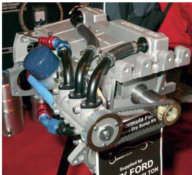
Left: new dry sump system from Pace Products designed for 1.6-litre Duratec engines used in Formula Ford
