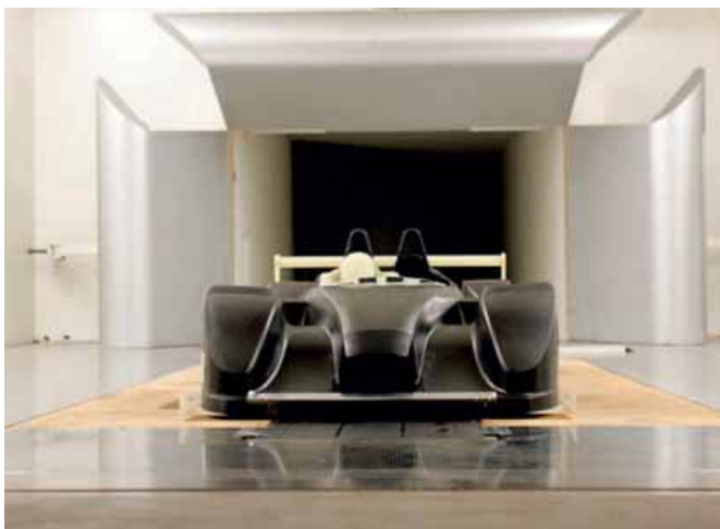
Wind tunnel work was done in both full scale and model tunnels at Weissach
