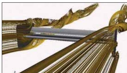
Figure 10 (right): end plates increase the effective aspect ratio by lessening the effect of the tip vortices (Advantage CFD)
