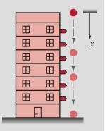
In terms of the coordinates shown in the figure (positive down), the speed of the ball v as a function of the distance x is given by  $v^2 = 2gx$ . Using linear regression, determine the experimental value of g.
