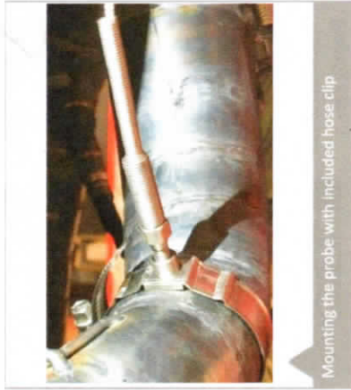
Mounting position: 15 cm distance to piston skirt
