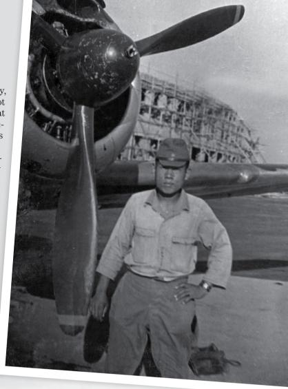
ABOVE: An unknown Army pilot poses with his Ki-43-II before deploying overseas. Note the starter spline on the central part of the spinner that was engaged to start the engine as required. Remote starters were mounted on trucks and drove a shaft mounted on a wooden A-frame to do the job.
