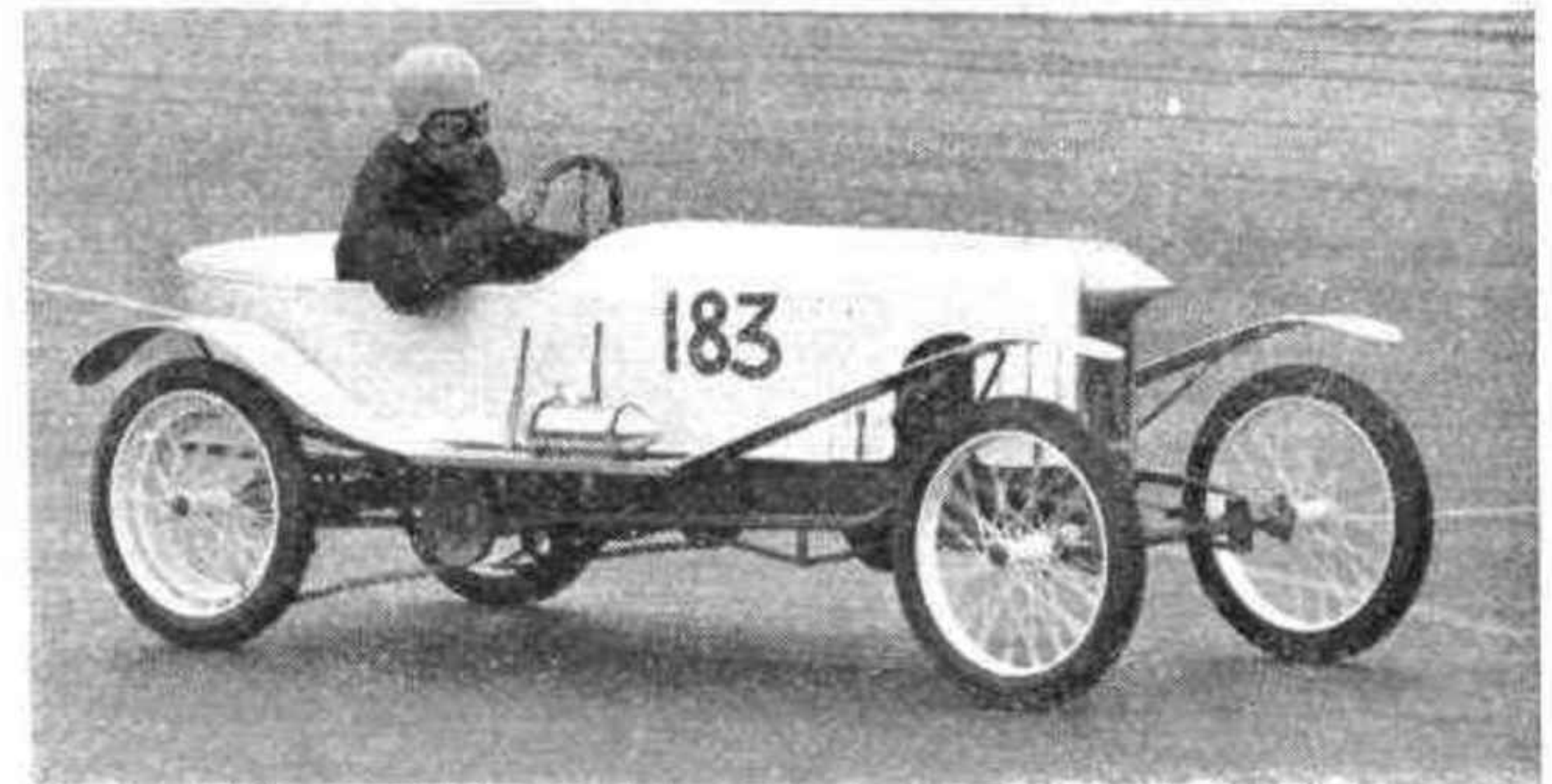
EDWARDIAN CYCLECAR. —A. R. Mitchell's 1914 GN was one of the attractions at the July VSCC Silverstone, driving belts flapping as it corners with determination. Note the "streamlined" tanks.
