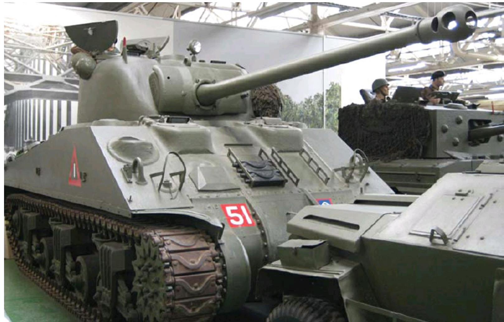
On display at the Tank Museum, Bovington, is a Sherman VC “Firefly” based on the medium tank M4A4. It is armed with a 17-pounder (76.2mm) main gun that proved to be one of the few Western Allies’ tank-mounted weapons that could penetrate the frontal armor of the German Panther tank at combat distances. (Tank Museum)
