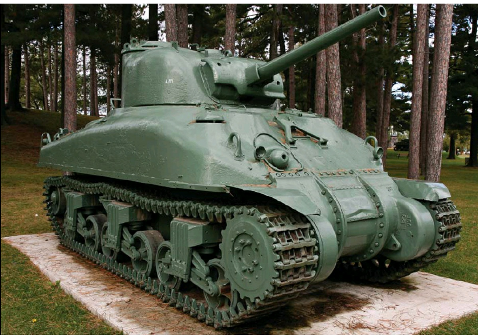
A Grizzly I medium tank on display at Base Borden in Canada. The Grizzly was essentially an M4A1 medium tank assembled by the Montreal Locomotive Works, and factory equipped to Canadian/British requirements. Due to production cutbacks in the M4 series medium tank program, only 188 units were produced from October through December, 1943. (Paul Hannah)
