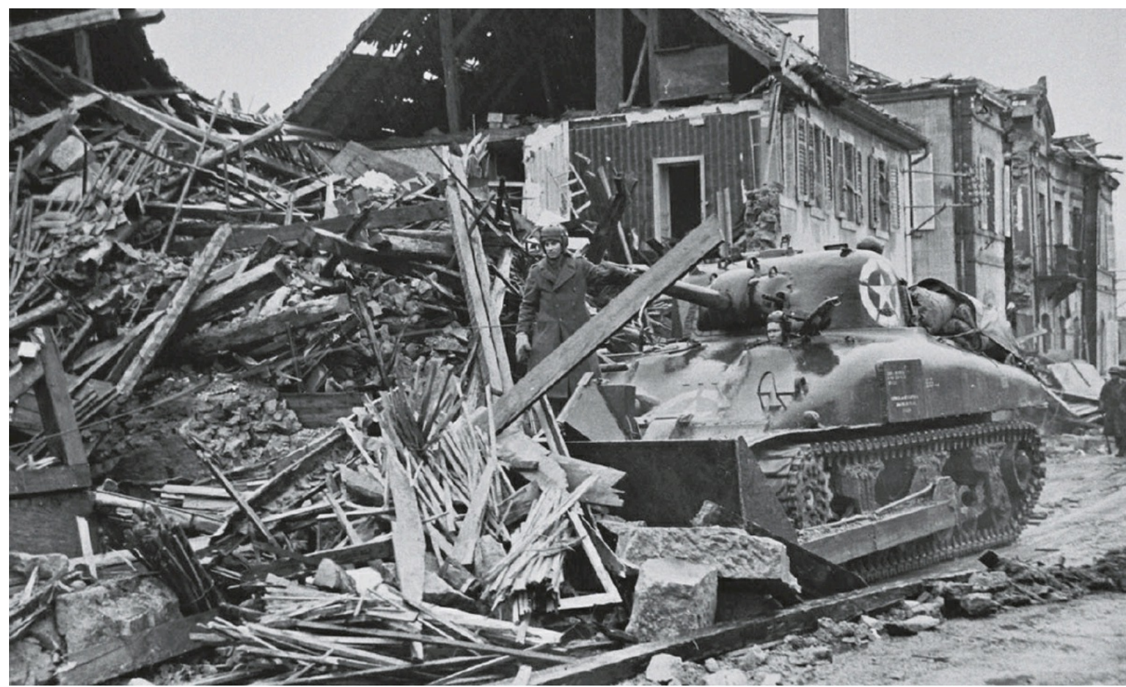
One of the most useful M4 series medium tank accessories was the tank-mounted bulldozer M1, seen here mounted on the front of a first-generation medium tank M4A1. Field expedient dozers had been used in 1943, but the M1 was first employed in Italy in spring 1944. (Patton Museum)
