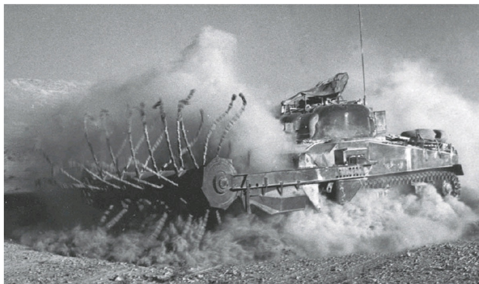
A medium tank M4A4 is seen here in postwar Israel Defense Forces service mounting a British-designed flail-type mine exploder, referred to as the "Crab II." When flailing, the Crab could only be operated at a maximum speed of 1.25mph. (Patton Museum)
