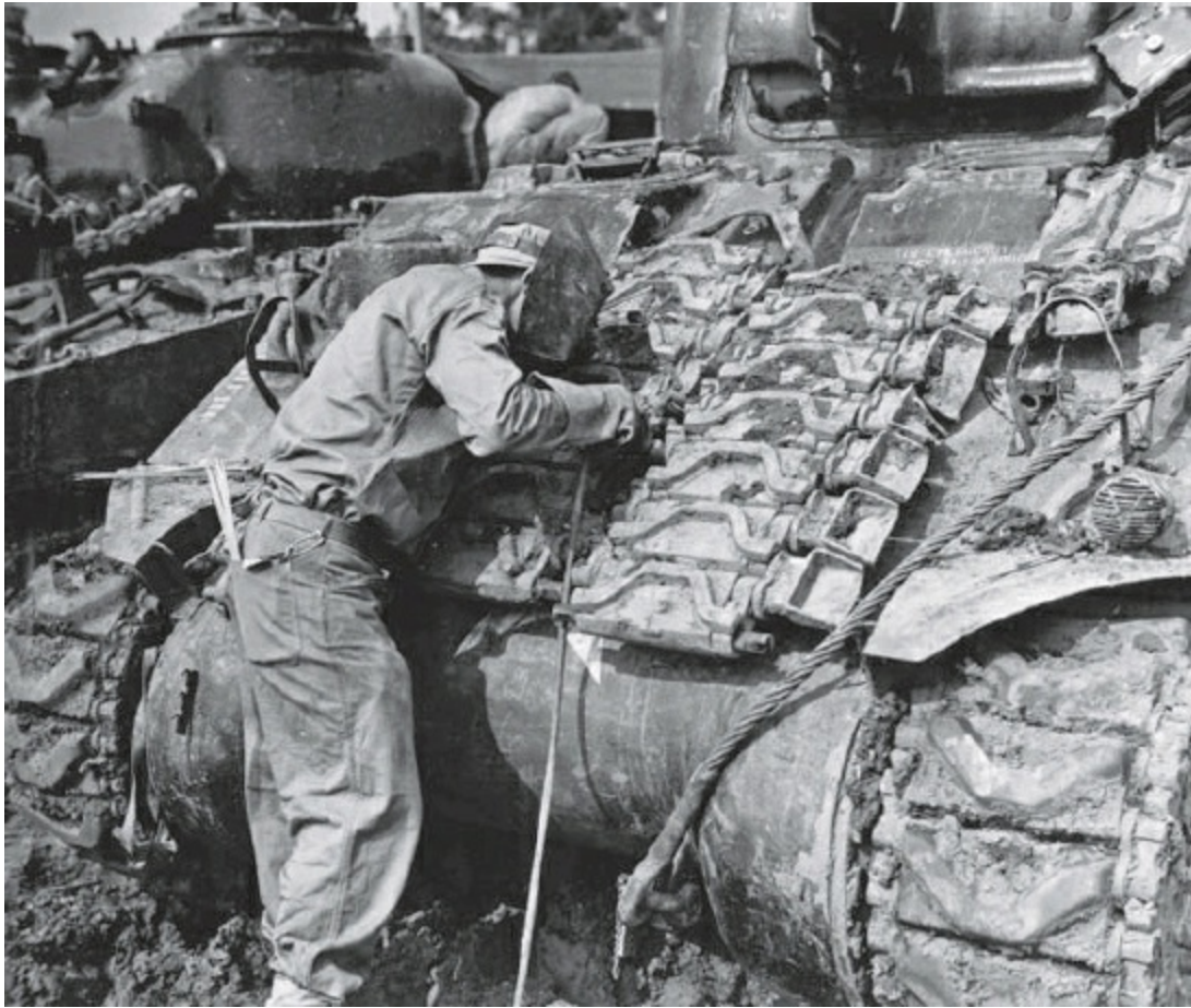
To increase the armor protection on their M4 series medium tanks, it was common for crews to weld spare track links onto the hulls as seen here. Sometimes the spare track links would also be welded onto the turret sides. (Patton Museum)
