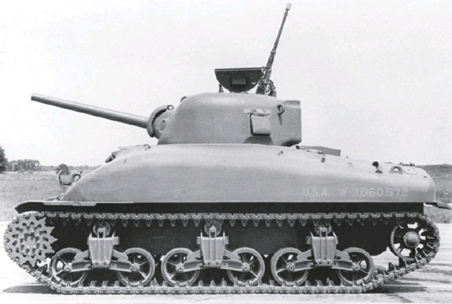
Pictured is the first medium tank M4A1 made by Pacific Car and Foundry. The VVSS was inherited from the M3 medium tank and can be identified by the return rollers mounted on the top of the bogie assemblies. Notice the pistol port on the left-hand side of the turret. (TACOM Historical Office)
