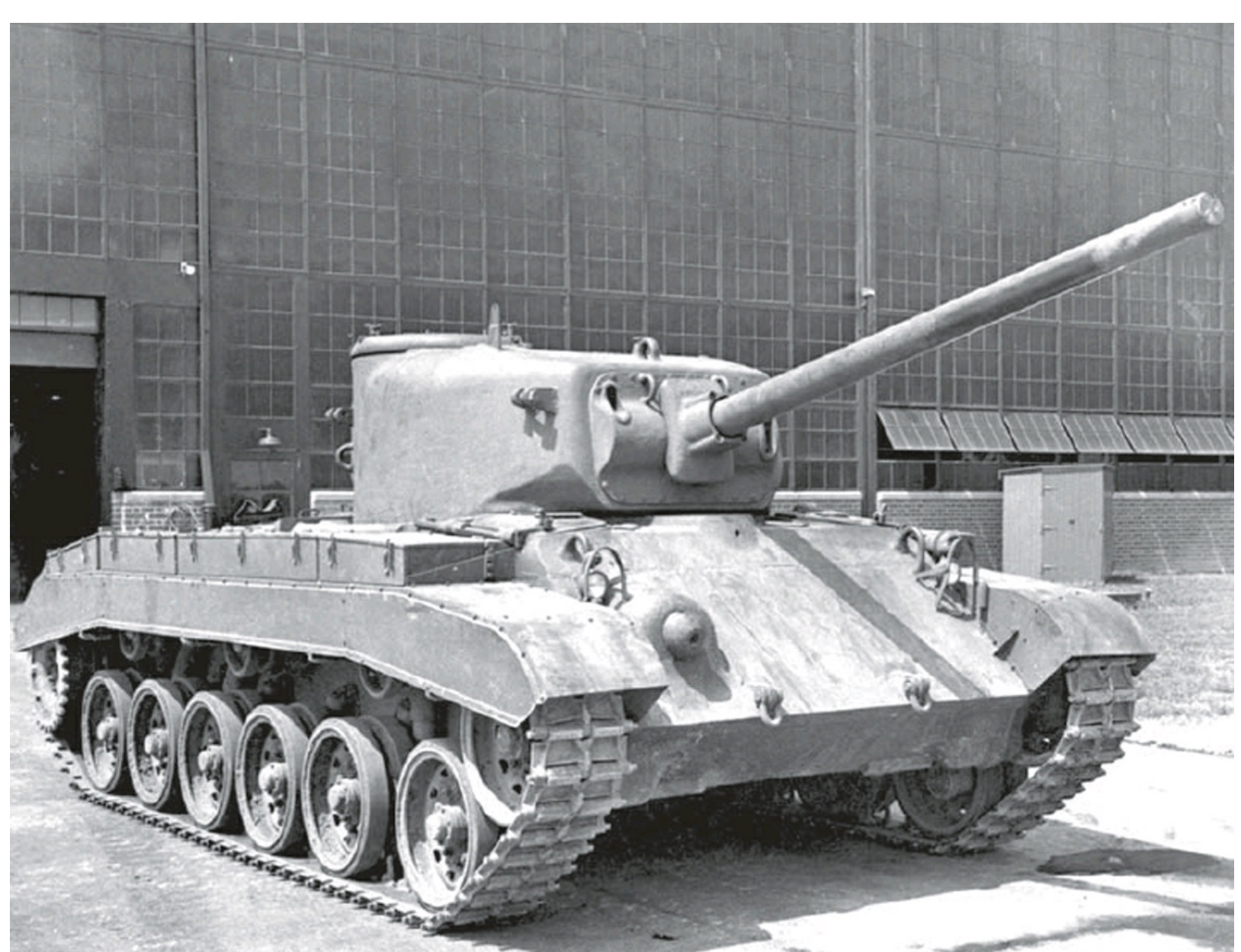
The T20 series of medium tanks was developed to replace the M4 series medium tanks. Pictured is the T20E3 pilot vehicle in July 1943. It was armed with a 76.2mm main gun and rode on a torsion bar suspension system. (TACOM Historical Office)
