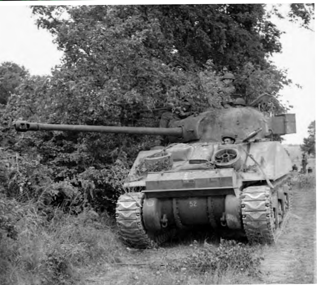
While no photos of Ekins's actual tank appear to exist, you can see the Firefly's main distinguishing feature from this image, the long barrel of its 17-pounder gun. The box-like extension to the turret rear accommodated radio equipment for which there was no longer any room in the turret proper.
