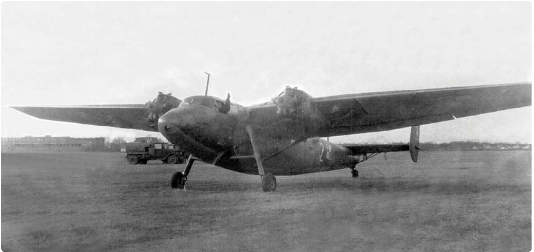
ABOVE Shcherbakov Shche-2 "White 2" has its engines run up in preparation for a training sortie while serving with the Polish Air Force's Military Pilots' School at Dęblin in eastern Poland circa 1946. Reportedly, while in V-VS service, one Shche-2 was fitted with General Motors diesel engines from an American armoured vehicle and flown.
