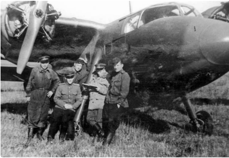
LEFT A rare photograph of a production Shche-2 (with M-11D engines and fixed-pitch two-bladed wooden propellers) at the V-VS Scientific Research Institute airfield, with a group of pilots and engineers. Second from right is test pilot and Hero of the Soviet Union Pyotr Belyasnik.
