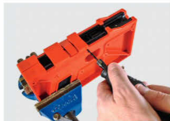
While it's recommended to use a drill press, Tarr was able to drill the pin holes in the P80 frame by hand with a Dremel tool.
