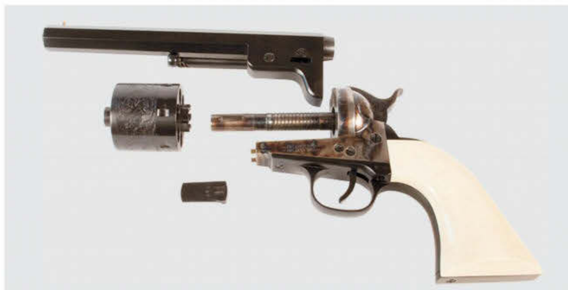
▲ Unlike Single Action Army-style revolvers, the 1851 Navy conversion's cylinder revolves on an arbor, and the barrel must be removed to pull the cylinder.
