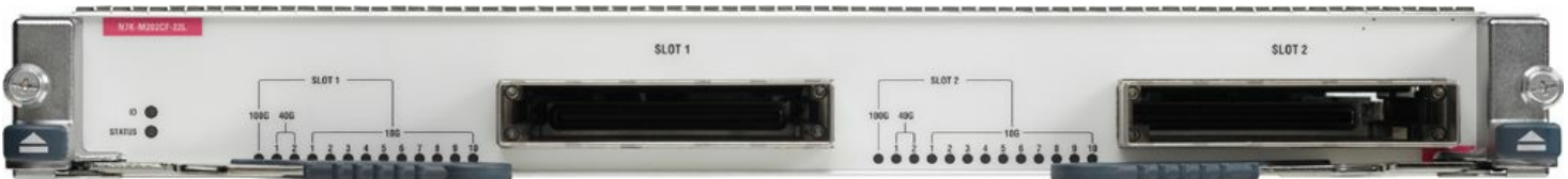
Figure 1-16. N7K-M202CF-22L – M2 Series 2-Port 100-G Module CFP Optics
