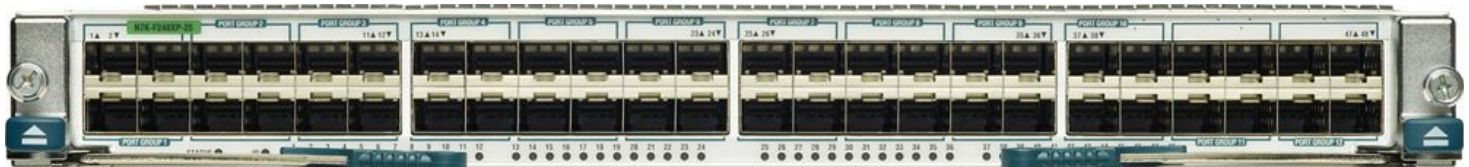
Figure 1-12. N7K-F248XP-25 - F2-series I/O Module 48-Port L2/L3 1/10GE SFP+ Module (req. SFP)
