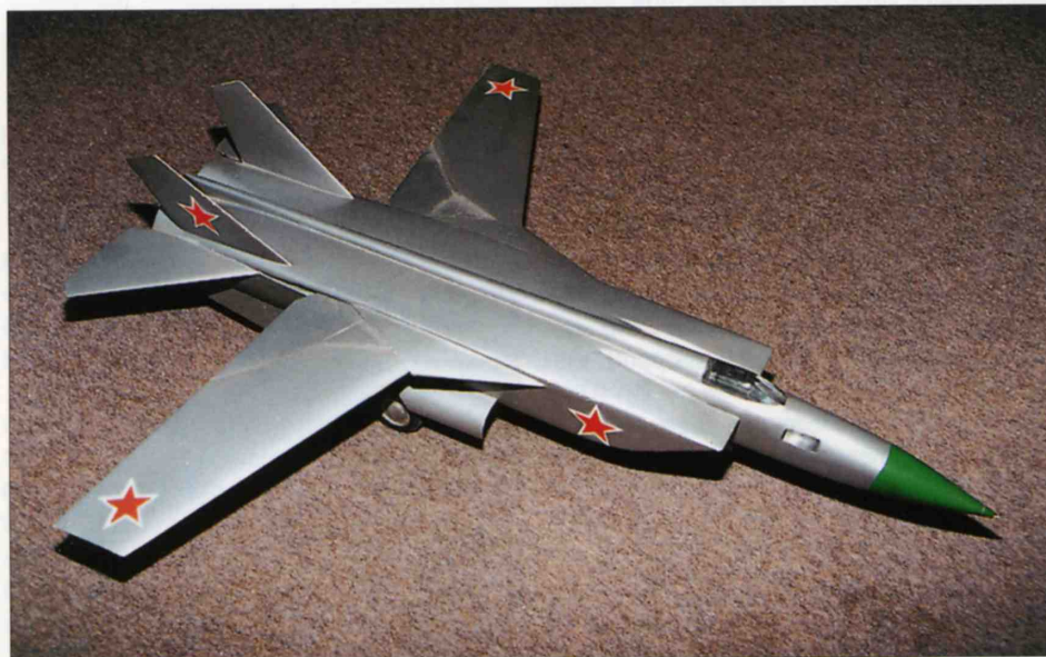
The same model with the wings at minimum sweep. Note the conical radome and the symmetrically located windows of the navigator's station aft of it. The small vertical tails are also noteworthy.
