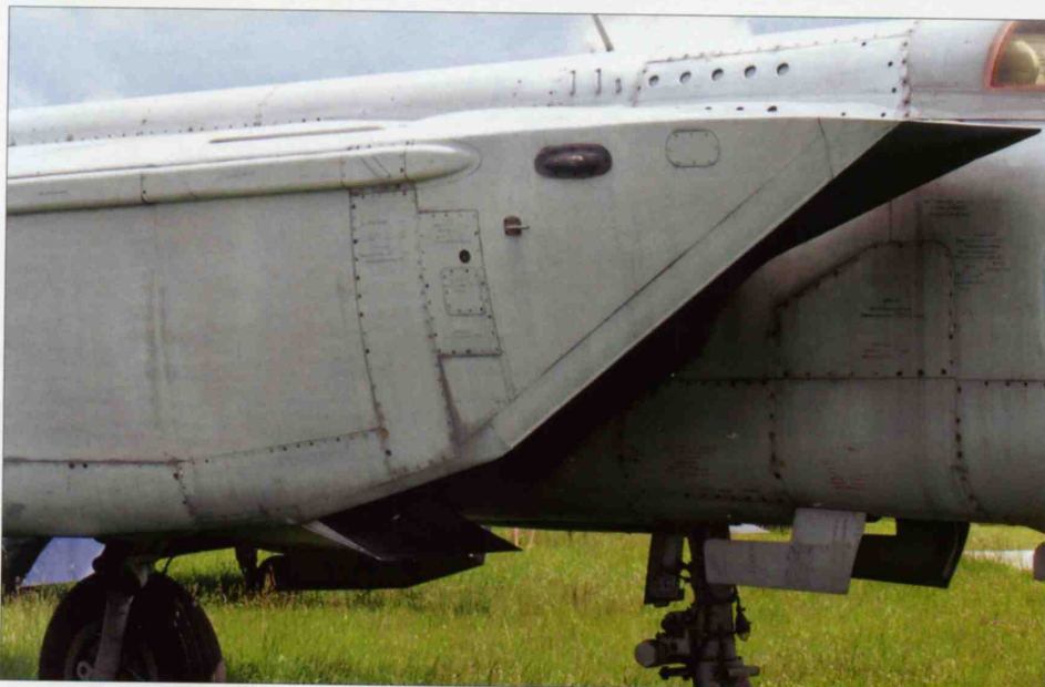
Above left and left: The air intake trunks feature removable panels (originally intended for access to the actuators of the canard foreplanes that were never fitted). Note the ECM antenna blisters.
