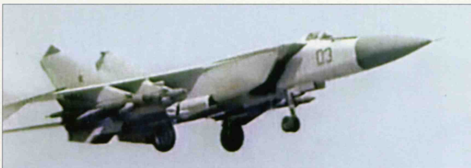
Above: '03 Red' (the Ye-155P-3) takes off with a full load of missiles. The wing endplates are just discernible.
