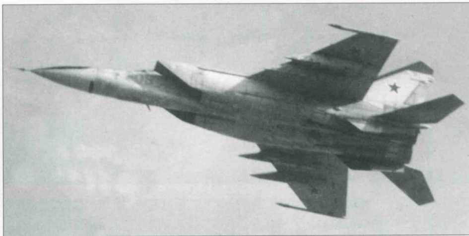
Above: MiG-25PD '305 Blue' after conversion under an unknown R&D programme. Note the metal nosecone replacing the dielectric radome.
