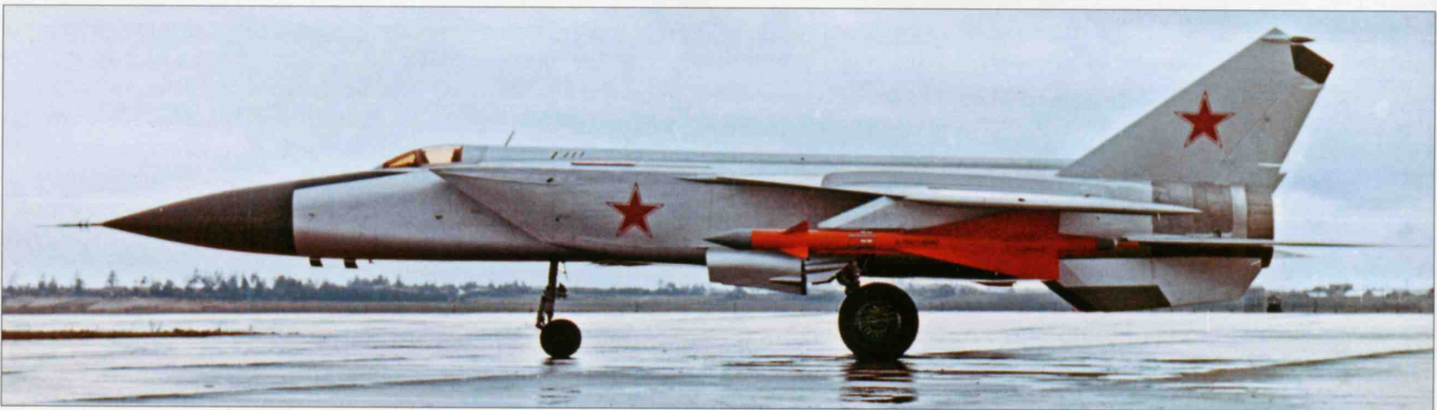
Three views of the Ye-155P-1 prototype fitted with a data link aerial and carrying inert K-40R AAMs on the as-yet two pylons. Note provisions for canards.
