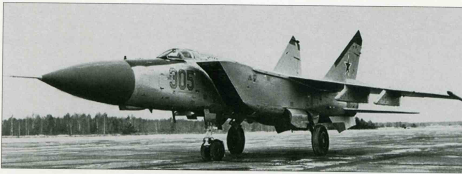
Above: '305 Blue', one of the MiG-25PD prototypes. The IRST fairing under the nose is clearly visible.
