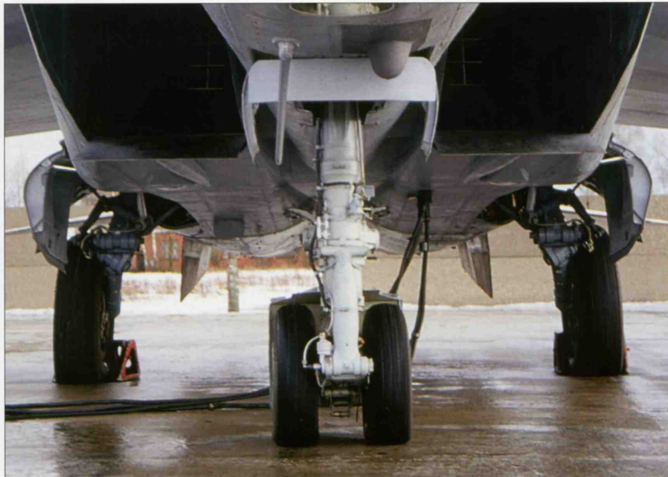
Left and above: The nose gear unit of a typical MiG-25 with a nose gear door segment doubling as a mud/snow/slush guard.
