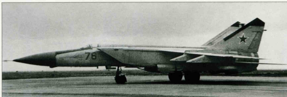
This MiG-25P coded '76' was a testbed for the Parol'-2 IFF system, as revealed by the small 'bump' below the radome.
