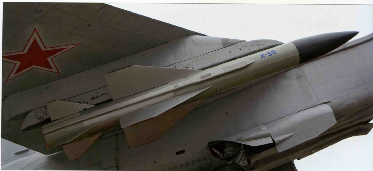
A Kh-58U anti-radar missile on an AKU-58 ejector rack fitted for show purposes to a MiG-25RBS preserved as a gate guard. This weapon is normally carried by the MiG-25BM.
