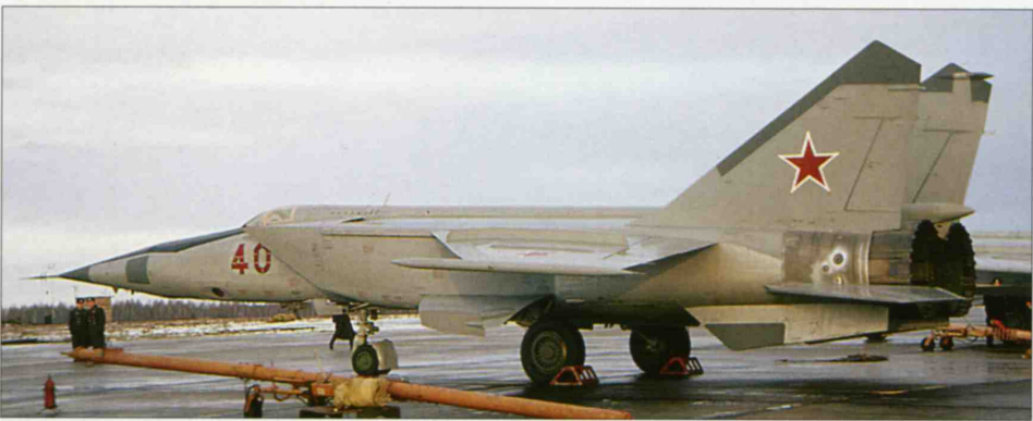
The later MiG-25RBT (illustrated by '40 Red', c/n N02008115 at Shatalovo AB) looks very similar to the MiG-25RBV, the late-style brake parachute housing being the main identification feature.
