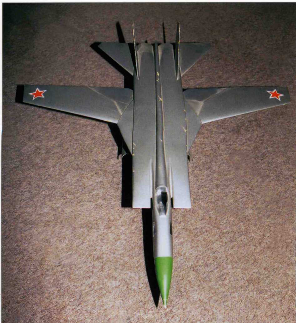
This upper view of the Ye-158 model shows that the wingtips were parallel to the fuselage centreline when the wings were fully deployed.
