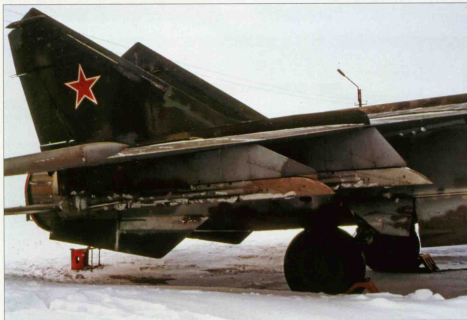
Top left: The original style of the brake parachute housing with a short pointed end.
