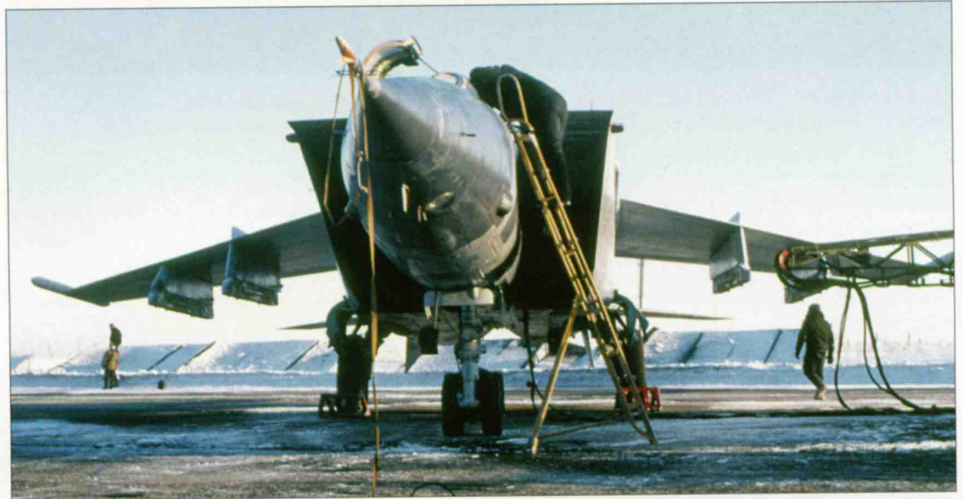
Above: This view shows clearly the MiG-25BM's four missile pylons fitted with AKU-58 missile adapters.
