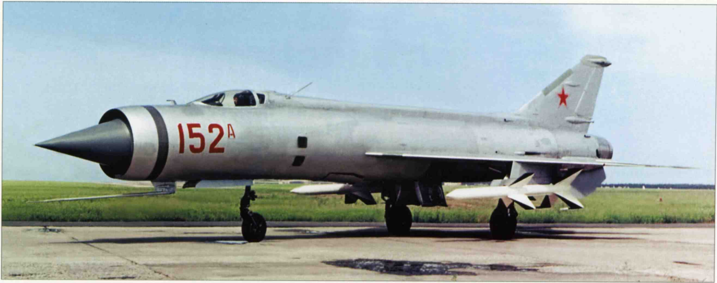
Above: The Ye-152A powered by two Tumanskiy R11F-300 turbojets was created as an insurance policy in case of possible development problems with the R15-300 engine. It carried the K-9-155 AAMs on underwing pylons.
