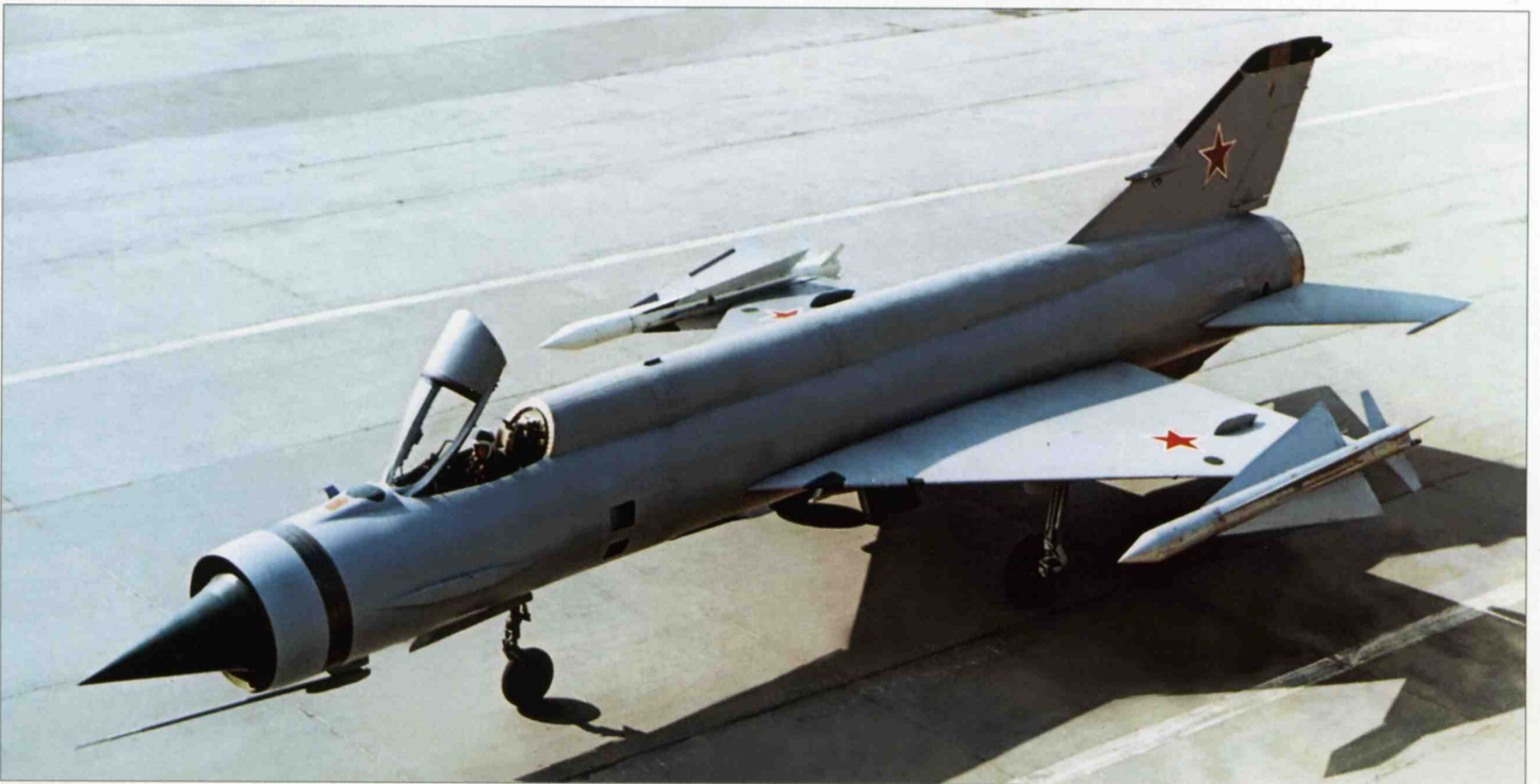
The Ye-152M – the ultimate development of the Ye-150/Ye-152 family – reverted to wingtip missile carriage but was armed with Bisnovat K-80 (R-4) AAMs. It also featured a fatter spine housing additional fuel, a revised cockpit canopy and provisions for canard foreplanes.
