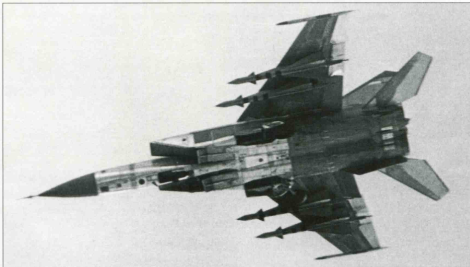
A brand-new MiG-25P makes a pre-delivery test flight in Gor'kiy. Though still unpainted and devoid of insignia, it carries dummy AAMs (to use a Russian jocular expression, it is 'trouserless but wearing a hat').
