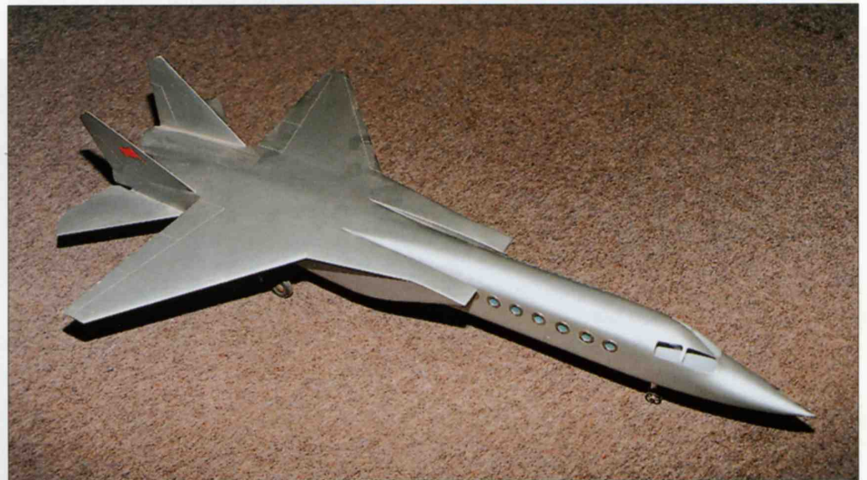
This view of the same model shows the modified wings of greater aspect ratio with LERXes and the large vertical tails.
