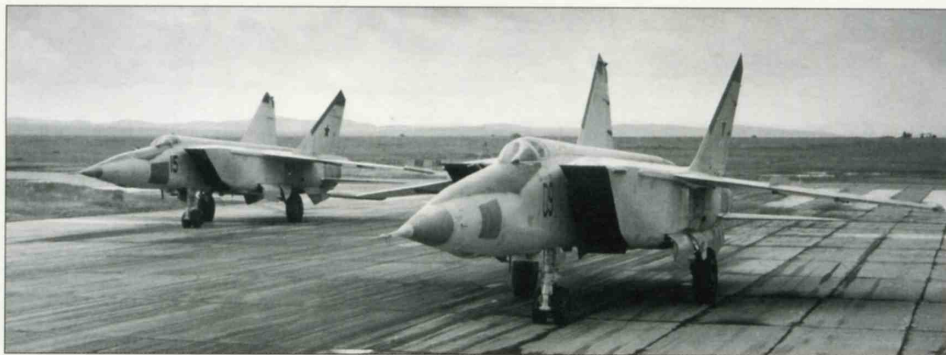
Above: A MiG-25RBK (right) and a MiG-25RBS line up for take-off. The different placement of the dielectric panels is obvious. Note the MiG-25RBK's enlarged dielectric nosecone.
