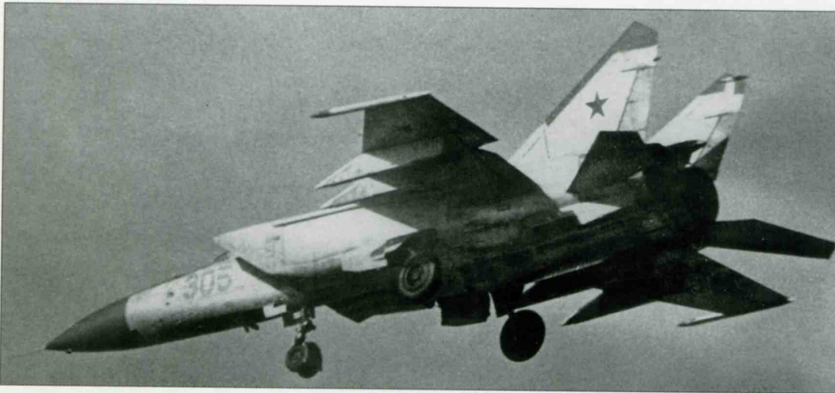
MiG-25PD '305 Blue' seen on final approach to Zhukovskiy. The aircraft has been modified for some test work (note the absence of the IRST).
