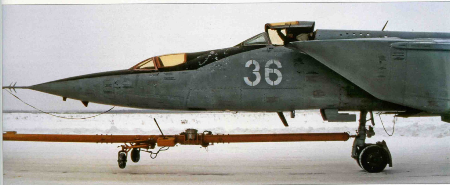
Another view of a trainer's forward fuselage (this time a MiG-25RU). The canopies open to starboard. With the nose gear unit positioned well aft, the MiG-25 requires a long towbar for ground handling.
