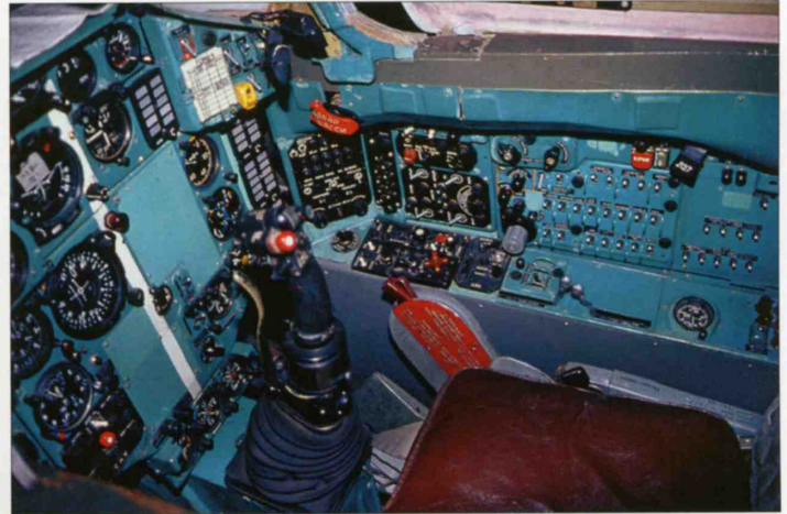
Two views of the cockpit of a MiG-25RB flight simulator. The lurid turquoise colour typical of Soviet aircraft is meant to reduce pilot fatigue.
