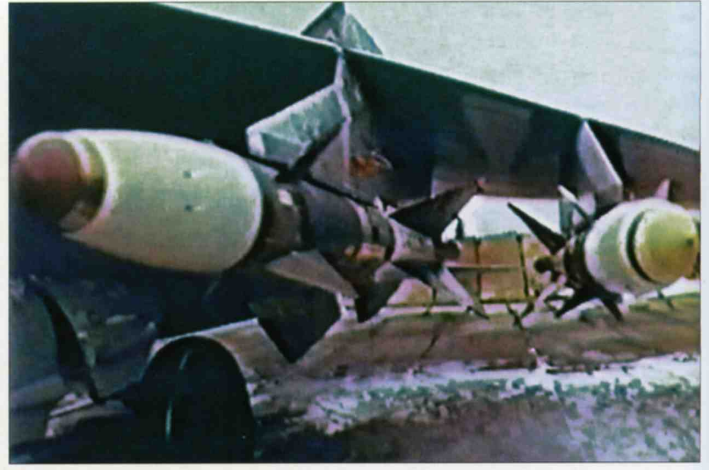
Left: A prototype K-40T medium-range IR-homing missile on a ground handling dolly. Right: A production R-40T (inboard) and a semi-active radar homing R-40R under the port wing of a MiG-25P.
