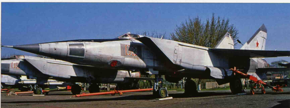
Above: MiG-25RBV '08 Red' is also used for instructional purposes at Tambov. This version reverted to small lateral dielectric panels positioned well forward.
