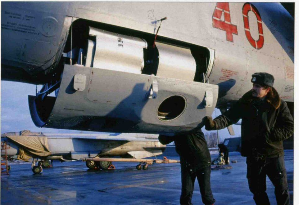
Top left: The underside of a MiG-25RBT's nose, showing the five camera ports.
