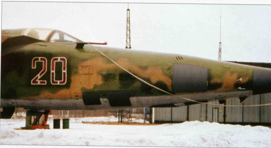
The MiG-25RBF has a similar nose shape but a large MiG-25RBK-style dielectric nosecone and additional dielectric panels low on the sides instead of camera ports.
