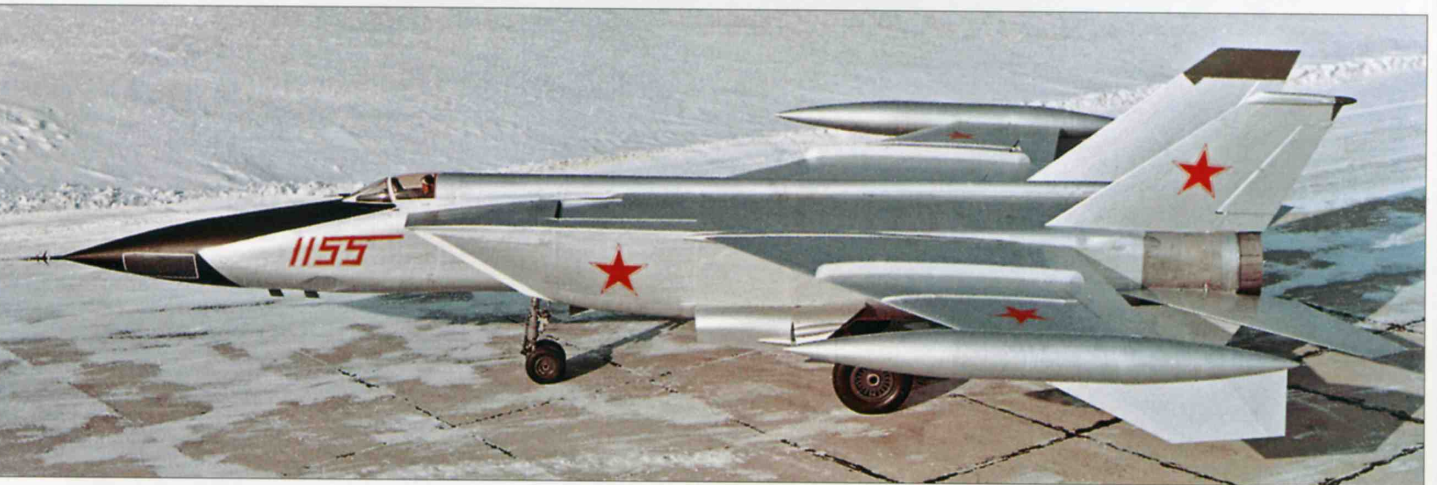
Four views of the Ye-155R-1 ('1155 Red'), showing the double-curvature nose with narrow dielectric panels, the tip tanks with downward-canted 'winglets', the horizontally cropped small fins, large ventral fins and low-set tailplanes. Note the closed nosewheel well doors and the star insignia on the fuselage.
