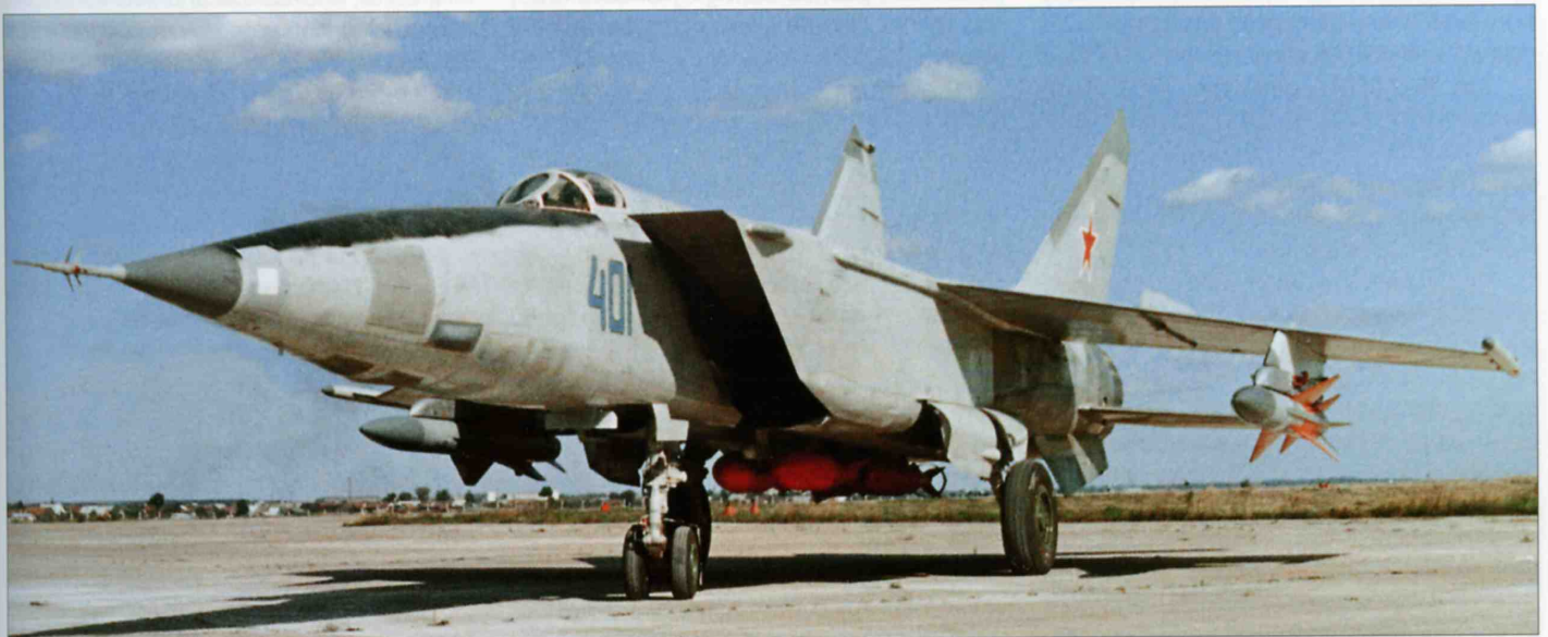
MiG-25RB '401 Blue' was one of several Foxbat -Bs modified under the MiG-25BM's development programme. The Kh-58U anti-radar missiles are well visible, as are the radar detection system antenna blisters low on the sides of the nose.
