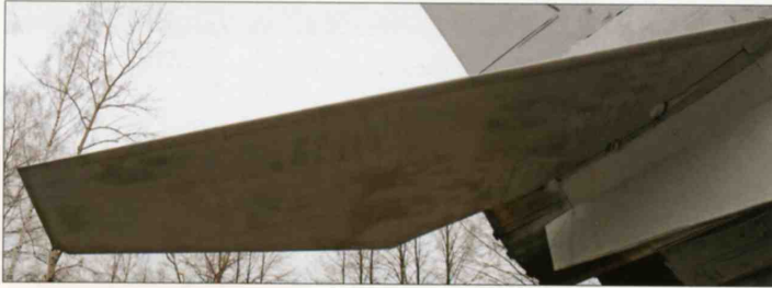
Left and above left: The MiG-25 has differentially controllable slab stabilisers; the tips are raked for better flutter resistance. Right and above right: The fins are augmented by trapezoidal ventral fins which incorporate dielectric portions enclosing more antennae.
