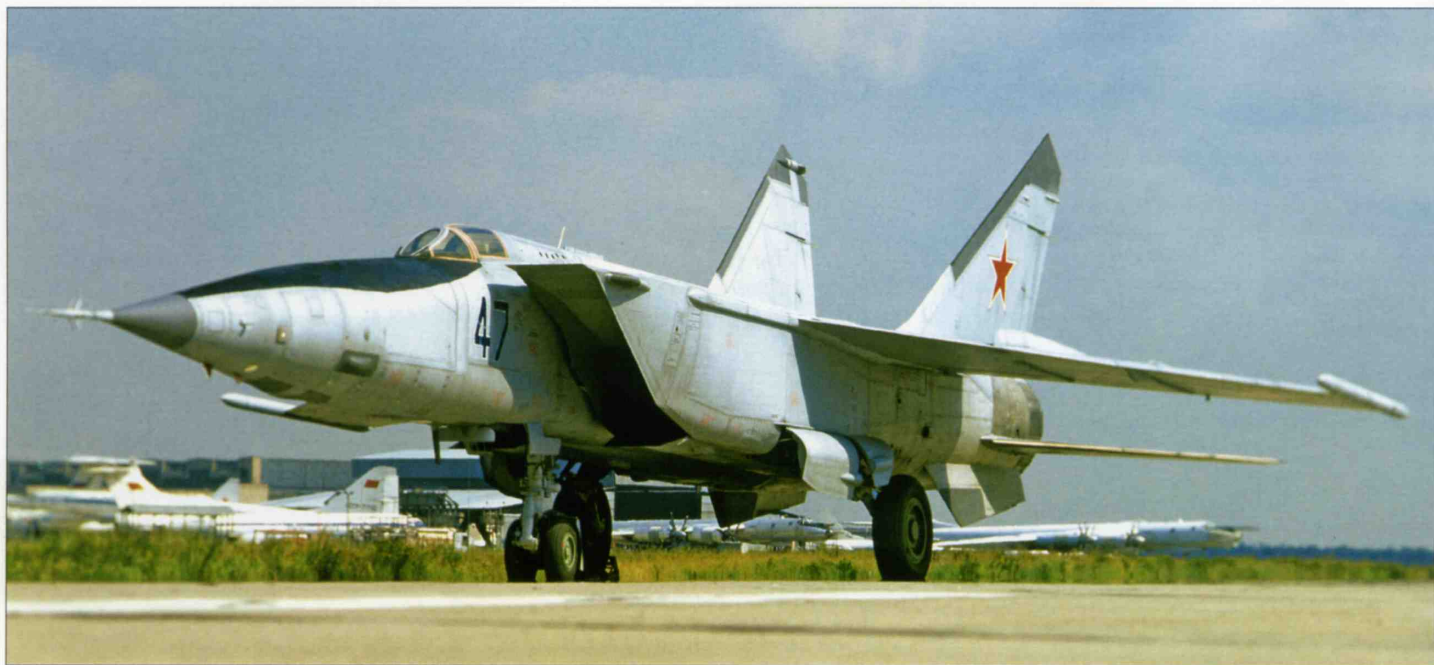
The penultimate step towards the creation of the MiG-25BM was the MiG-25RBM development aircraft. It is seen here at parked Zhukovskiy after transfer to LII.
