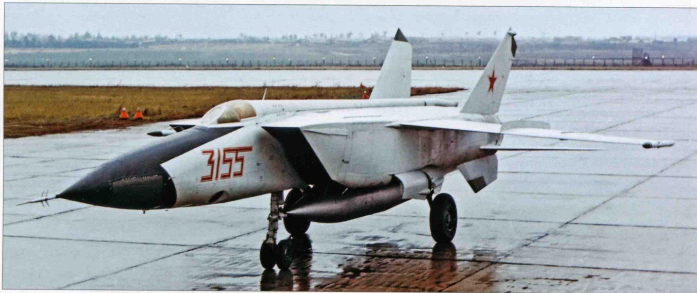
Three views of the Ye-155R-3, showing the lack of tip tanks (replaced by anti-flutter weights), the functional camera ports and the relocated data link aerial.
