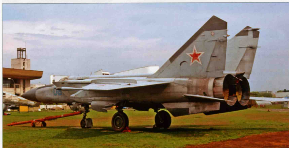
MiG-25PDS '08 Blue' (c/n N84018081) on display at the open-air museum at Moscow-Khodyinka. This view shows the original short brake parachute housing that was retained after the PDS upgrade.
