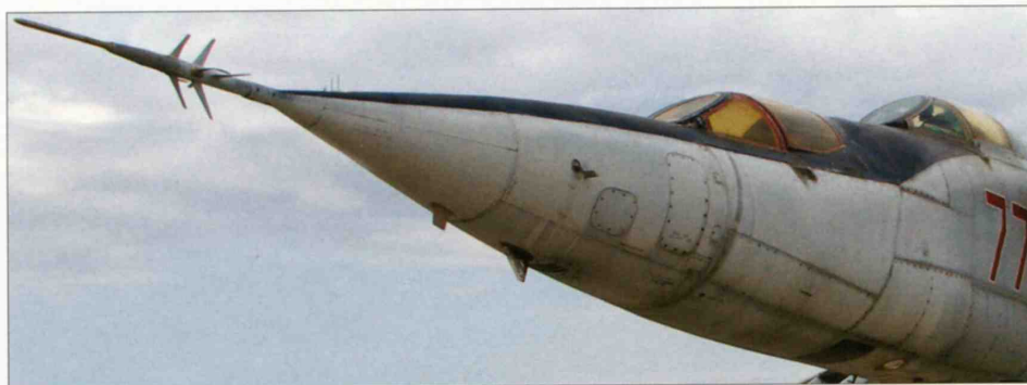
Above: The forward fuselage of a MiG-25PU, showing the stepped-tandem cockpits and the all-metal nosecone.
