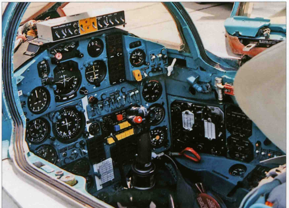
The front cockpit of the same aircraft. Note the special control panel on top of the instrument panel.
