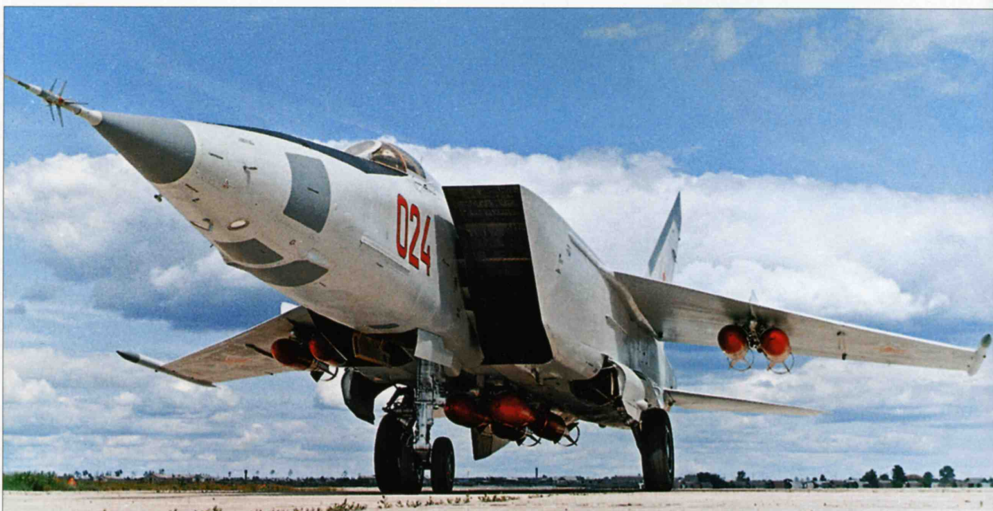
'024 Red', the MiG-25RB prototype (Ye-155R-4B), with a full load of eight FAB-250M-62 low-drag bombs. The aircraft has the original nose gear door design but has been retrofitted with wingtip anti-flutter weights.
