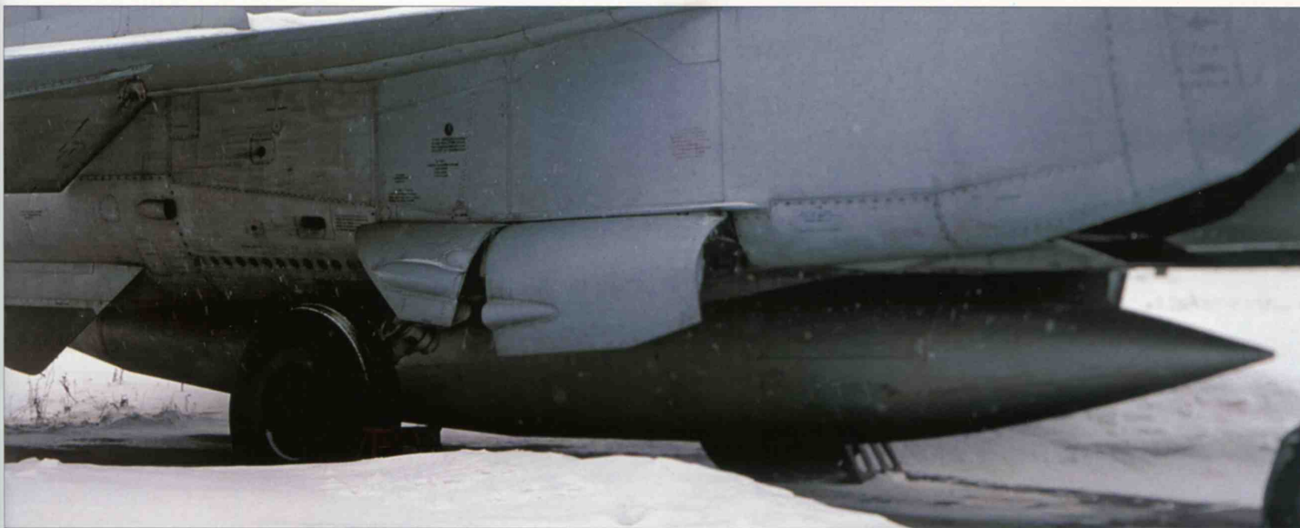
Above: The 5,280-litre drop tank suspended beneath a MiG-25RB. Note the short pylon at the front.
