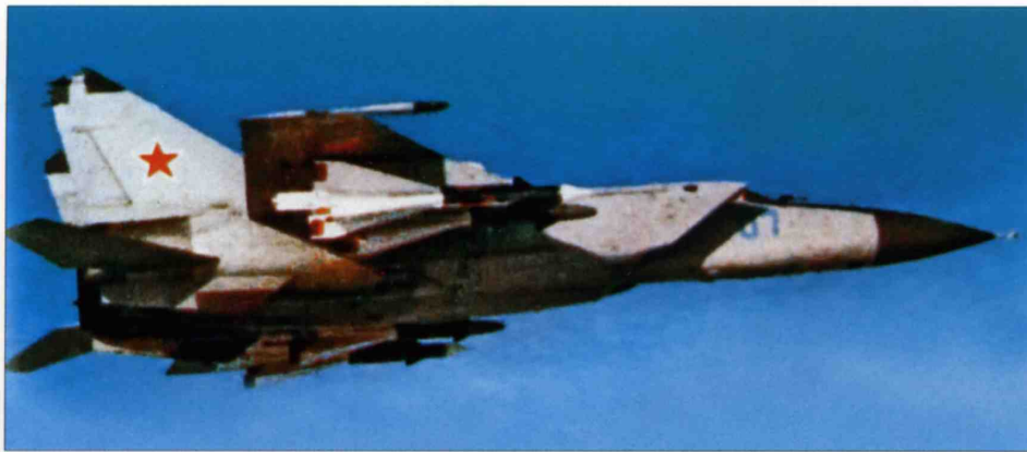
'07 Blue', an operational Soviet Air Force MiG-25P, toting a typical ordnance load – two IR-homing R-40Ts inboard and two semi-active radar homing R-40Rs outboard.
