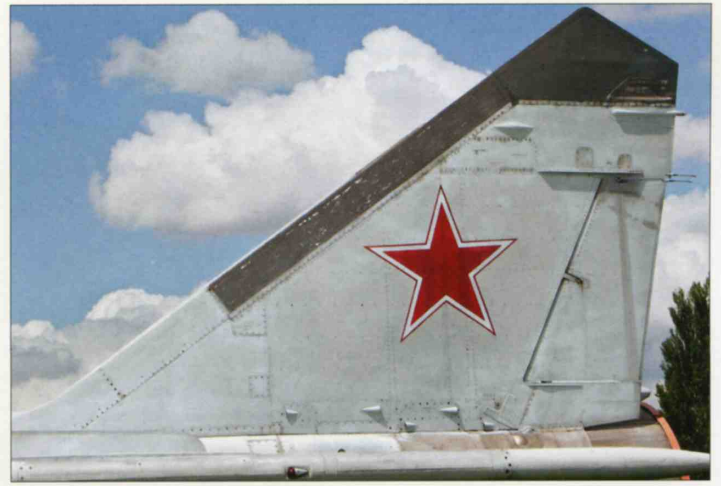
Above, left and right: The fins of the MiG-25 incorporate various navigation and communications antennae. The configuration of the dielectric portions on the port and starboard fins differs.
