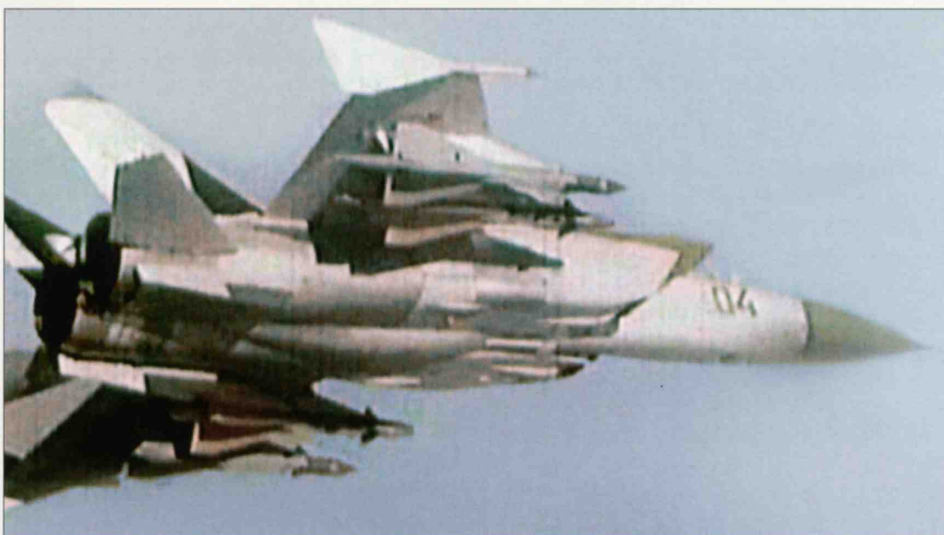
The Ye-155P-4 ('04 Red') breaks formation with the camera ship, showing the ventral fairing housing test equipment.
