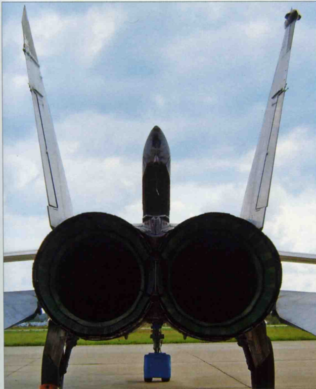
Left: The fins of the MiG-25 are canted slightly outward. Note the open brake parachute housing. Right: The tail unit of a MiG-25PD.
