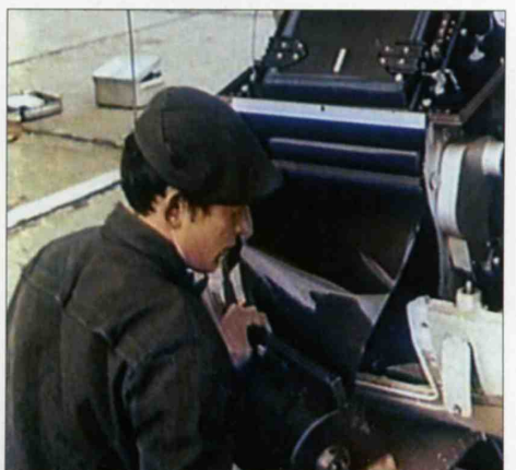
Top right, above left/right and below left: Lowering the camera pallet of a MiG-25RBT at Shatalovo AB. The hinged covers provide access to the retaining bolts.
