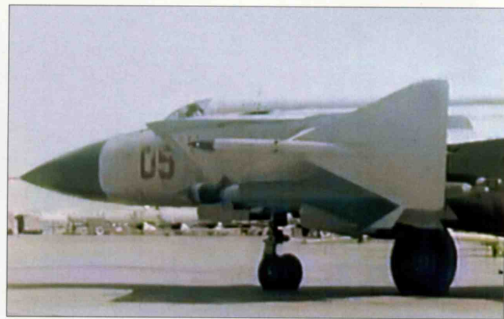
Above, left and right: Showing signs of wear and tear, the Ye-155P-5 taxis with K-40T heat-seeking missiles on the pylons during the State acceptance trials. The port air intake carries four 'kill' stars denoting successful test launches. Note that the large ventral fins have been replaced by the definitive tapered version.
