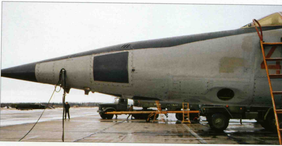
Above: The nose of the MiG-25RBT is similar to that of the MiG-25RBV – unsurprisingly, since only the equipment inside is different. The forward camera ports are hard to spot from this angle.
