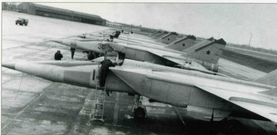
A MiG-25RBS heading a line-up of reconnaissance/strike MiG-25s shows off its characteristic large dielectric panels concealing SLAR antennas.
