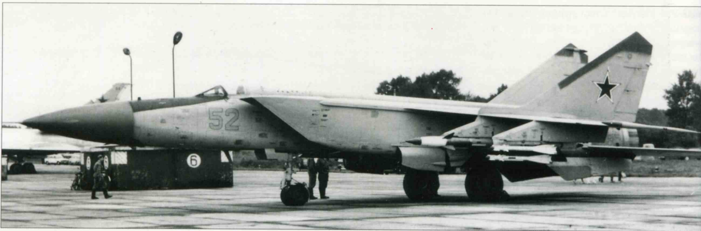
Above: '52 Blue', an operational MiG-25PD armed with two R-40RD medium-range AAMs and four R-60M short-range AAMs on twin adapters.
