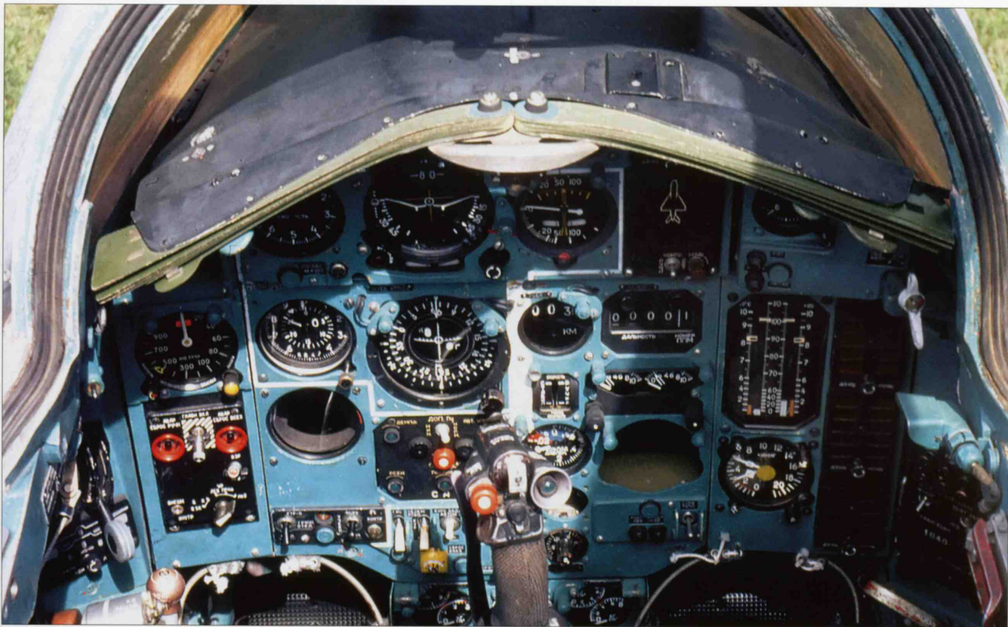
Above: The main instrument panel of a MiG-25BM SEAD aircraft. The basic instrumentation is somewhat different (in particular, the vertical strip gauges for the engines on the right are noteworthy).
