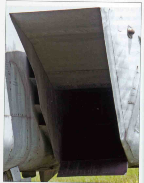
Top left: The port air intake of a MiG-25PD. Note the protective sheath on the lower intake lip preventing injuries to ground personnel.
