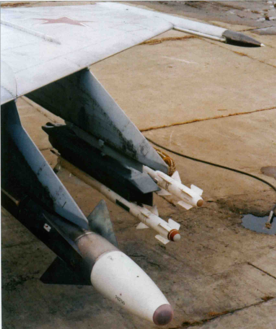
Above: An R-40TD and two R-60M short-range IR-homing AAMs on an APU-60-2 paired launcher under the port wing of a MiG-25PD.
