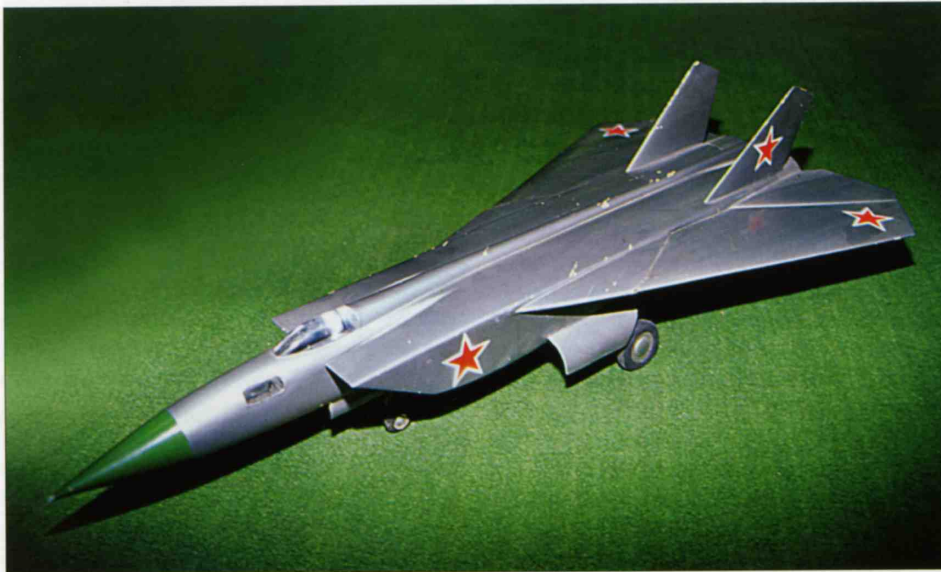
Above: The Ye-158 model with the wings at maximum sweep. Note how the wings effectively form a common lifting surface with the tailplanes set high up on the fuselage.
