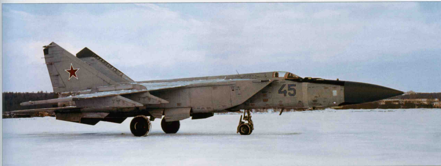
'45 Blue', the MiG-25PDZ in-flight refuelling system testbed. The retracted IFR probe is just visible ahead of the cockpit.
