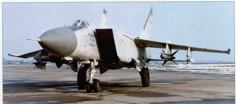
Two views of '306 Blue', another MiG-25PD prototype. Note the black anti-glare panel ahead of theIRST.
