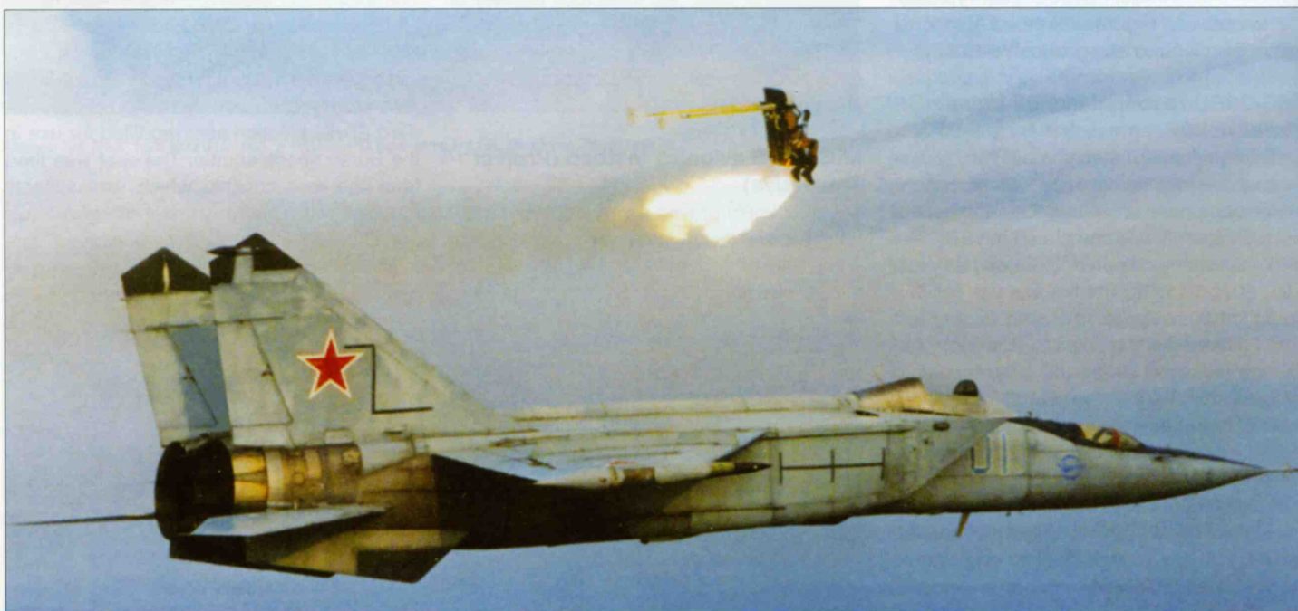
Seen here with the new tactical code '01 Blue' and the LII logo on the nose, the testbed fires a Zvezda K-36RB ejection seat. The seat's distinctive stabilising booms tipped with drogue parachutes are deployed.
