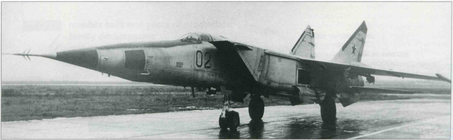
Above: MiG-25RBK '02 Blue' (c/n N02029210) served as an avionics testbed under the Buran space shuttle programme. Note the rectangular dielectric panel on the air intake trunk.
