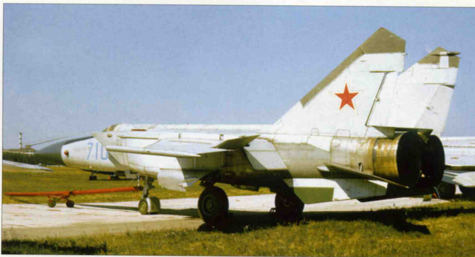
Above: '710 Blue', one of the two 'MiG-25M' development aircraft, in the open-air museum at Moscow-Khodynka. The 'solid' nozzle shrouds of the R15BF2-300 engines are well visible from this angle.
