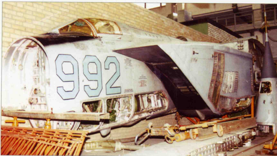
The remains of the second izdeliye 99 engine testbed ('992 Blue') serve as a teaching aid at the Moscow Aviation Institute. Note the nose section on the right clearly indicating the machine's MiG-25R lineage.
