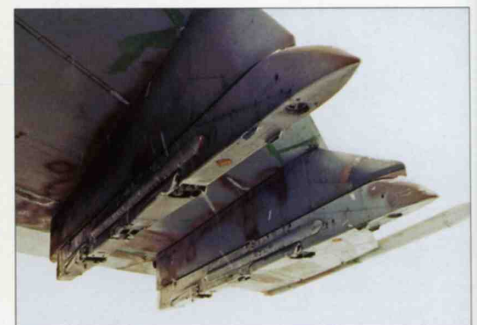
Left and below: The pylons of a MiG-25BM fitted with AKU-58 ejector racks.
