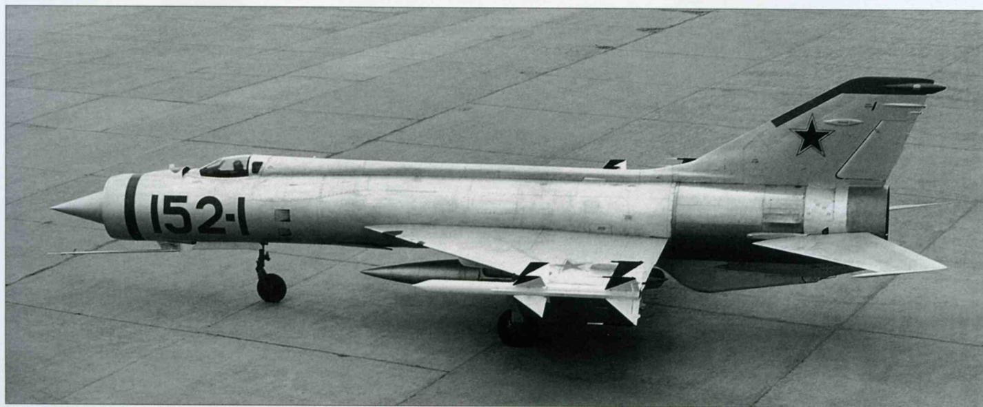
The appropriately marked first prototype of the single-engined Mikoyan/Gurevich Ye-152 all-weather heavy interceptor, shown here with centreline drop tank and two Mikoyan K-9-155 missiles on wingtip launch rails. Though ill-starred, the Ye-152 helped greatly to develop the future MiG-25 – in particular, its powerplant.
