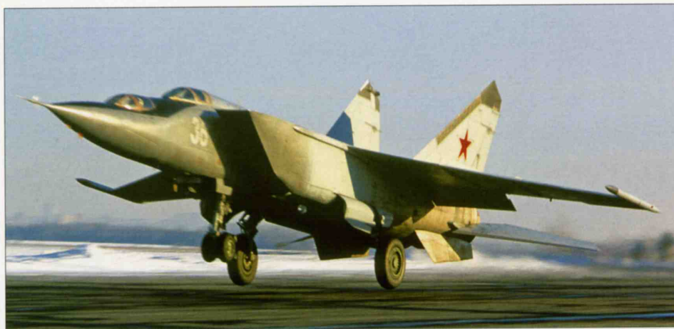
A Russian Air Force/4th TsBP i PLS MiG-25RU takes off from Lipetsk-2 AB, showing the lack of pylons.
