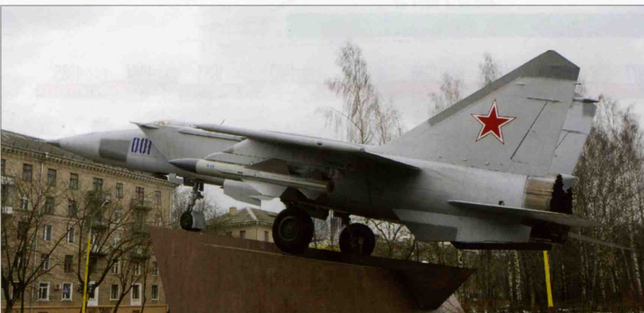
The same aircraft preserved in front of the MKB Raduga weapons design bureau in Doobna, Moscow Region, wearing the spurious tactical code '001 Blue' and sporting Kh-58U anti-radar missiles on MiG-25BM style pylons under the wings.
