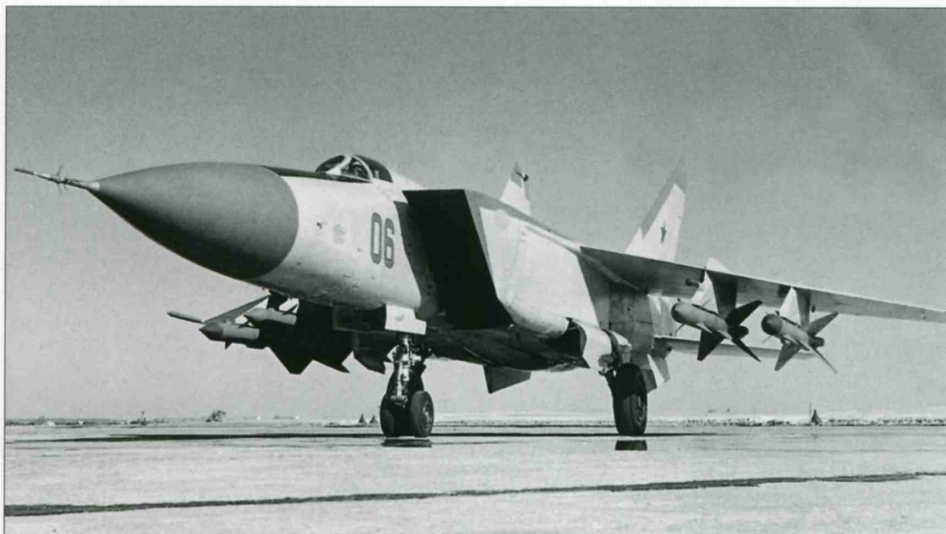
Left: '06 Blue', the Ye-155P-6 development aircraft, was the first MiG-25 to feature the production-standard large vertical tails.
