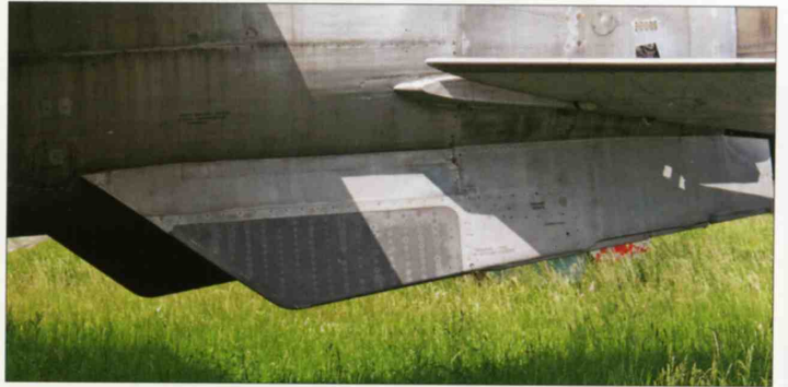
Left and above left: The MiG-25 has differentially controllable slab stabilisers; the tips are raked for better flutter resistance. Right and above right: The fins are augmented by trapezoidal ventral fins which incorporate dielectric portions enclosing more antennae.
