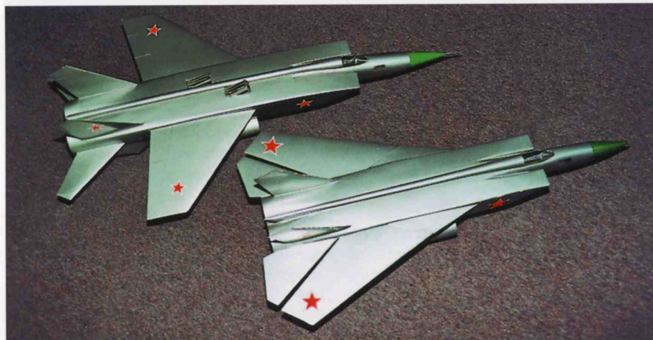
Top: A model showing a proposed STOL version of the Ye-155R with tandem lift-jets.
