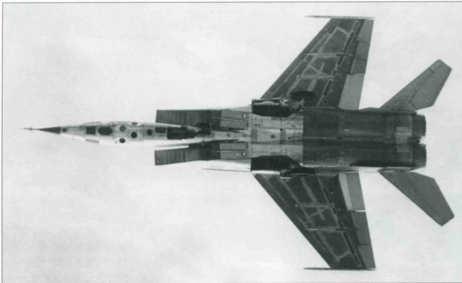
A brand-new and still-unpainted MiG-25RB makes a test flight from Gor'kiy, showing off the camera ports.
