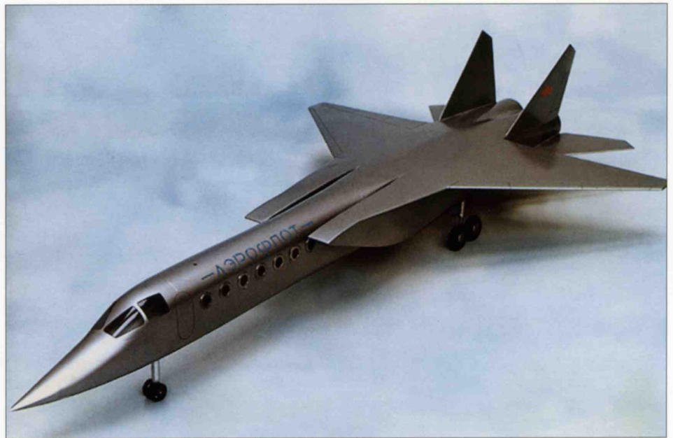
Above: A model of the proposed supersonic business jet derivative of the Ye-155 showing the all-new forward fuselage and main gear units. The number of cabin windows appears too large.
