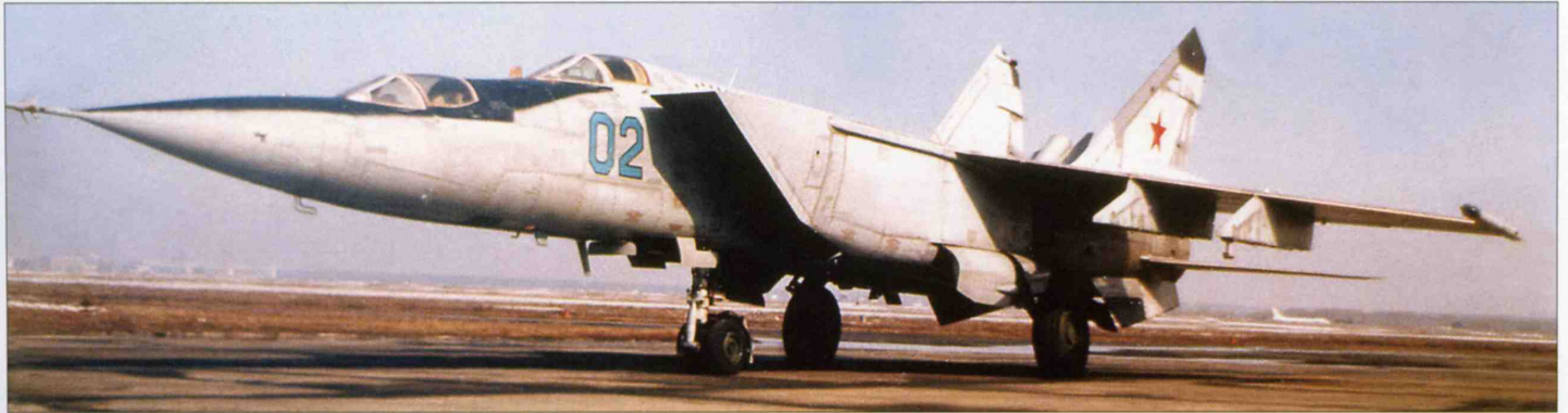
Above and below: '02 Blue', the MiG-25PU modified for verifying the Buran space shuttle's control system. It is seen here at Zhukovskiy, its home base.
