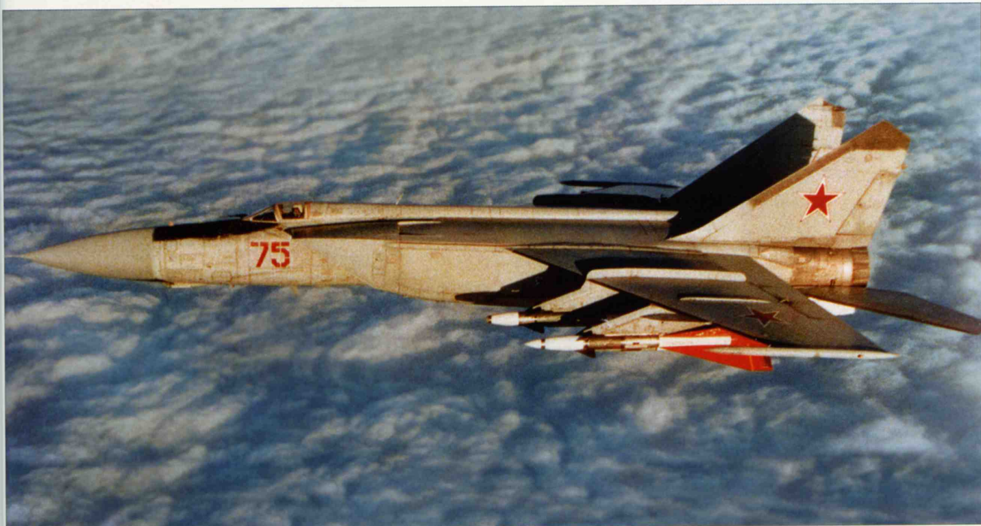
This overall view of a MiG-25PD flying above heavy overcast shows clearly the aircraft's layout with massive air intake trunks flanking the forward fuselage to blend into the centre fuselage.
