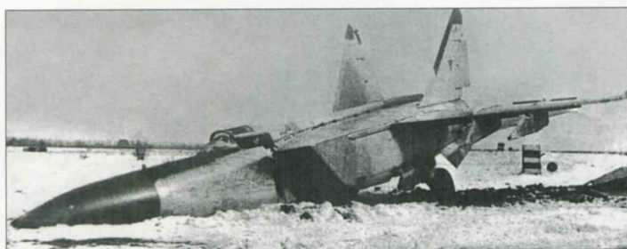
Left and above left: This MiG-25P coded '42 Blue' overran the runway when returning home from a practice sortie and was totalled, collapsing the nose and starboard main gear units and snapping the fuselage in the cockpit area. Note that the brake parachutes were not deployed.
