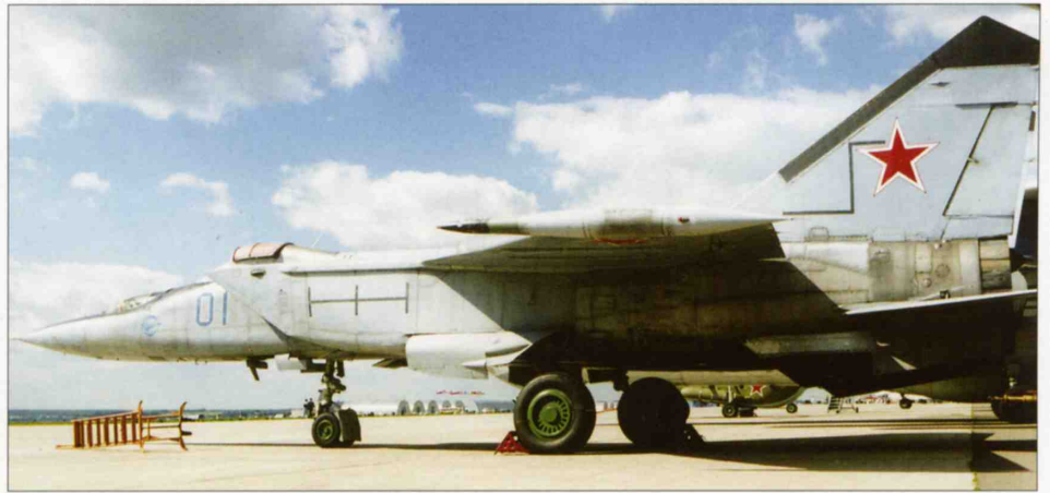
Above: Here the ejection seat testbed has a special cover placed over the rear cockpit. Note the non-standard fat wingtip pods.
