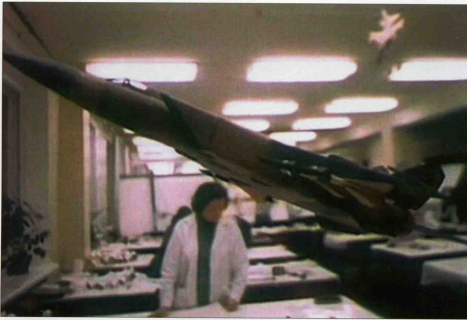
Above: An early model of the Ye-155P interceptor. Note the four K-40 AAMs under the wings.
