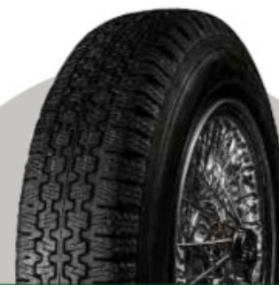
PIRELLI CINTURATO CA67 The original sports car radial tyre, from the 1950s through the '60s and into the '70s. As fitted to the DB4 GT Zagato Borrani wheel - THE works upgrade for '50s and '60s DB models.
