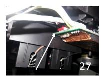
Take the other end of the audio cable with Red connector and connect it to the sound board of the PT01S
