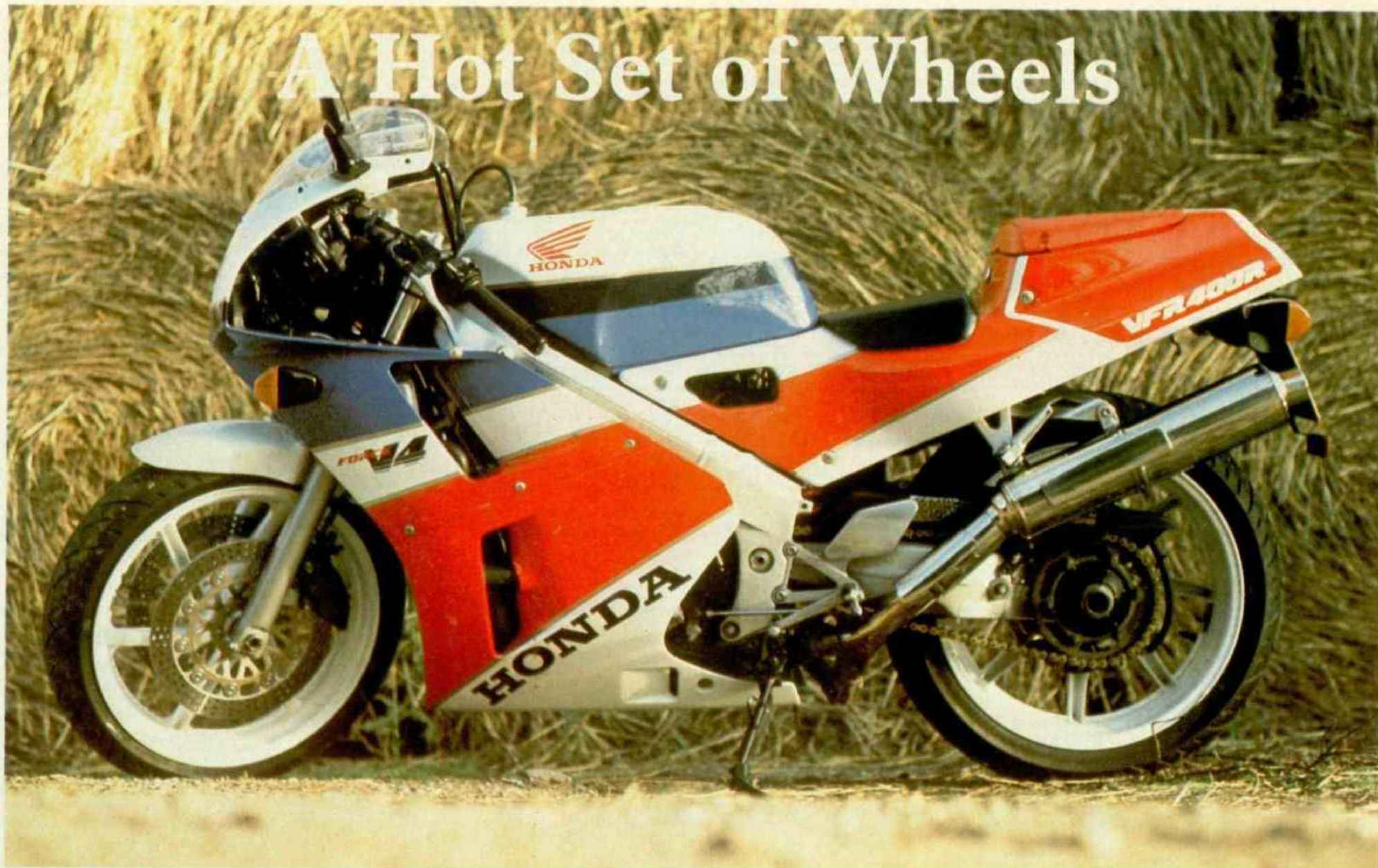
The race replica Honda VFR400R – a 400cc four-stroke that can rev up to 15,000 rpm!
