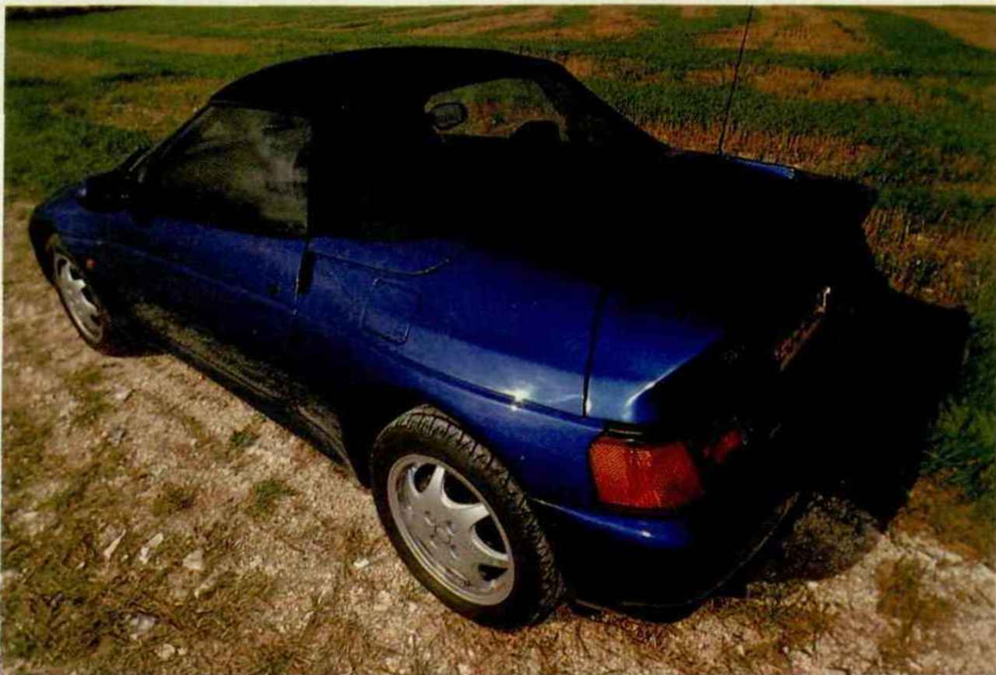
The unlined hood is easy to erect, but it does cause a certain amount of loss of rear vision.
