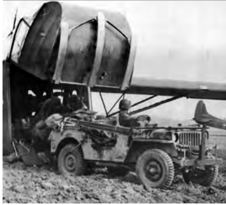
ABOVE: A jeep exits a CG-4A through the hinged nose fitted with Corey skids. Warner's glider carried a jeep that had to be abandoned on the landing zone due to intense German fire. BELOW: Tom Warner's good friend, Curtis J. "Goldie" Goldman—brash, cocky, and fearless—stands with a Thompson submachine gun slung over his shoulder on a Varsity LZ.
