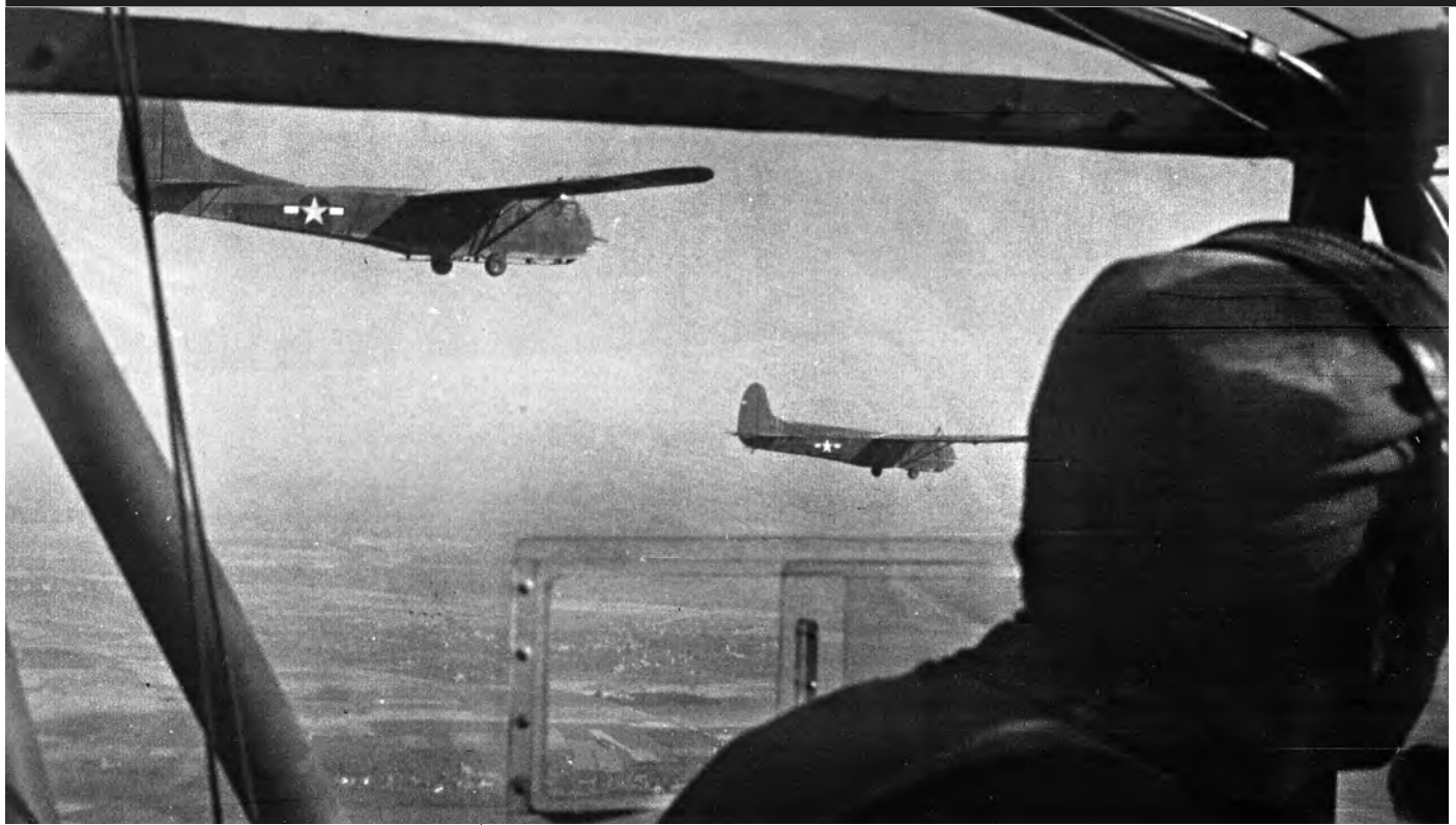
Two CG-4A Waco gliders, being towed by a single C-47, approach the release point near Wesel. Each Waco could carry 13 soldiers, a 75mm howitzer, a jeep, or a 1/4-ton trailer; 906 American gliders took part in Varsity.
