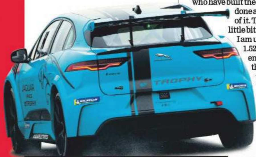
The I-PACE has an adjustable rear wing
