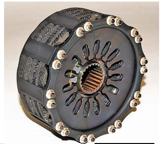
An F1 clutch weighs 1kg and measures less than 10cm
