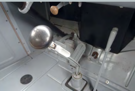
Gear lever, foot controls - without a synchro, gear changes aren't the smoothest
