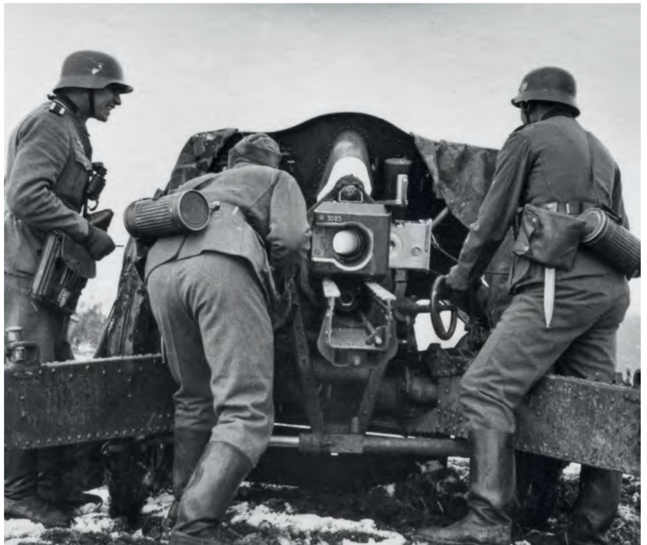
This view shows the divided responsibilities for traversing and elevating the leFH 18. K1 (Kanonnier 1, Gunner 1) stands to the left of the breech, and aims and traverses the gun. K2 stands on the right, and elevates the gun. K2 also fires the gun by pulling on a lanyard attached to the firing lever on the right-hand side of the breech block. The breech is open in this view (KRIEGSBERICHTER GUT.JAHR)
