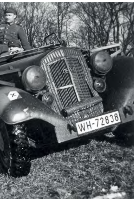
ABOVE: Kübelwagen served in an leFH 18 battery in various roles. One of these was as a signals car (Nachrichtenkraftwagen Kfz 15). Identification is by the telephone cable reel mountings on the front wings. (The designation was originally Fernsprechkraftwagen -Field Telephone Car). This one is based on a Horch 830 R, evidently built before 1936 as it has canvas instead of steel doors RIGHT: This leFH 18 is being towed by a five-tonne semi-track Sd Kfz 6/1. The vehicle is painted in a dark grey/dark brown camouflage pattern (B MITSCHÉ) BELOW: First time on the range for this 10,5 cm leFH 18 battery
