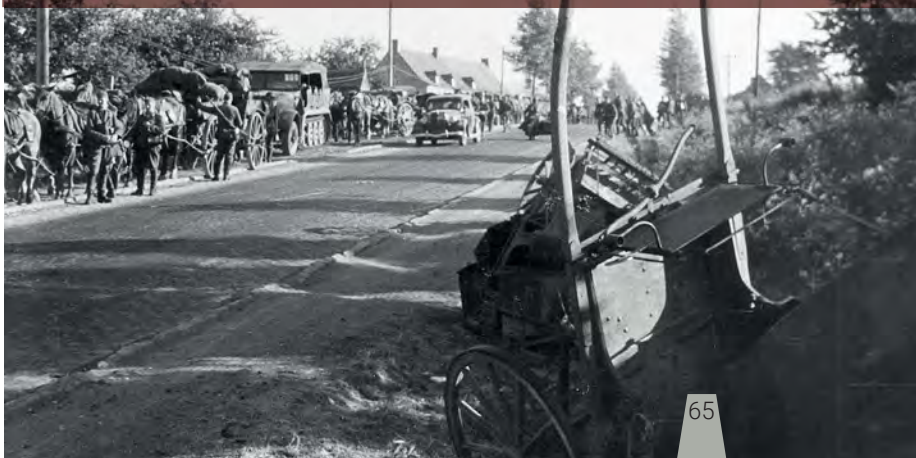
A horse-drawn artillery battery pauses by the side of the road; it looks like France or the Low Countries in 1940. Nearest the camera is a Beobachtungswagen (Observation Wagon), which, as well as its crew, carries an observation ladder, telescope, rangefinder etc. Next is a five-tonne semi-track (Sd Kfz 6/1). Why it is issued to a horse-drawn battery is not known; it may be for use in recovering guns from muddy firing positions. Behind the semi-track is an leFH 18, hauled by the standard six-horse team. Passing the battery is a 1935 Ford, impressed from its civilian owner for use by the military
