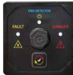
GAS DETECTION 12/24 VDC 2-5/8 in. (76 mm) Square Current Draw @ 12 VDC: 40 mA One Integral Sensor
