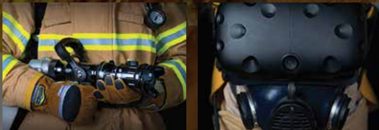
Force feedback supplied through hose to simulate water force. HTC VIVE virtual reality immersive headset.
