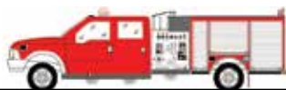
DARLEY VISION INITIAL ATTACK IA005 (CAFS Option Included) Pump (1000-1500) 300 Gallon Tank Copolymer Attack Body
