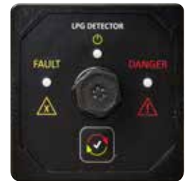
PROPANE DETECTION 12/24 VDC 2-5/8 in. (76 mm) Square Current Draw @ 12 VDC: 40 mA One Integral Sensor
